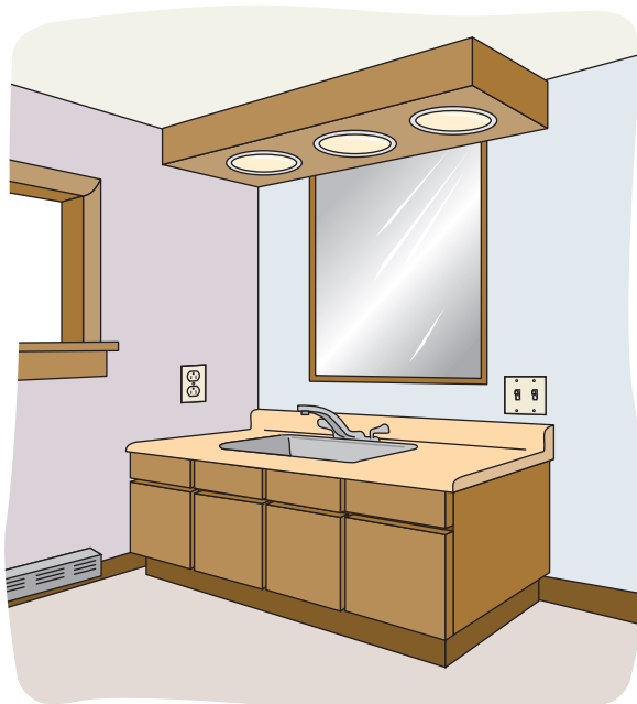
Typical incandescent recessed soffit lighting over bathroom vanity
