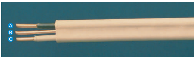
FIGURE 4-10 A nonmetallic-sheathed Type NM-B cable showing (A) black “ungrounded” (hot) conductor, (B) bare equipment “grounding” conductor, and (C) white “grounded” conductor.
