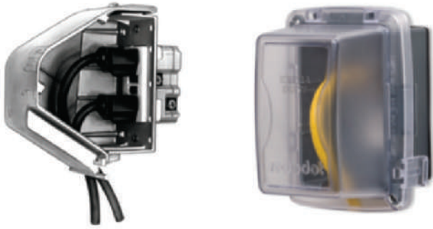
FIGURE 16-7 Weatherproof receptacle covers are required to be marked “Extra Duty.” They are available in metallic and nonmetallic types. Straight blade receptacles rated 15 and 20 amperes, 125 through 250 volts, installed in wet locations, must be listed as weather-resistant type.
