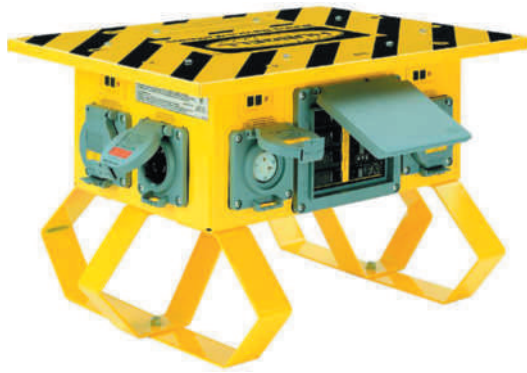
FIGURE 6-24 A temporary power box used on construction sites. This particular type is connected with a 50-ampere, 120/240-volt power cord. It has six 20-ampere, GFCI-protected, 125-volt receptacles plus additional 30-ampere and 50-ampere Twist-Lock receptacles.
