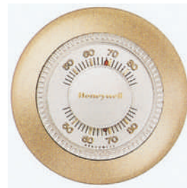
FIGURE 23-2 Thermostats for electric heating systems. A thermostat or other switching device that is marked with an OFF position must open all ungrounded conductors of the circuit when turned to the OFF position. Typical mounting height is 52 in. (1.3 m) to center.
