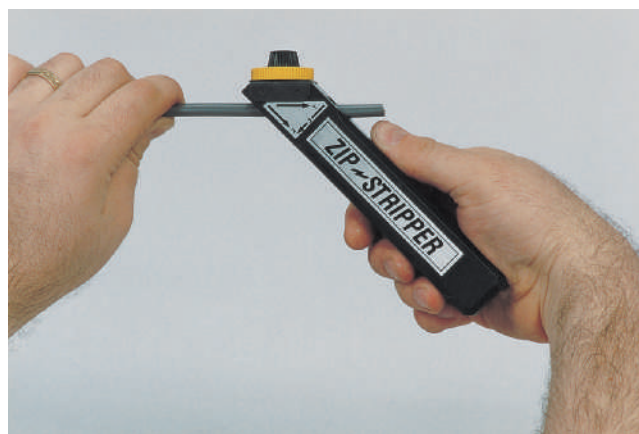
FIGURE 4-11 This stripper is used to remove the outer jacket from nonmetallic-sheathed cable.
