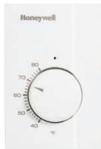
FIGURE 23-2 Thermostats for electric heating systems. A thermostat or other switching device that is marked with an OFF position must open all ungrounded conductors of the circuit when turned to the OFF position. Typical mounting height is 52 in. (1.3 m) to center.
