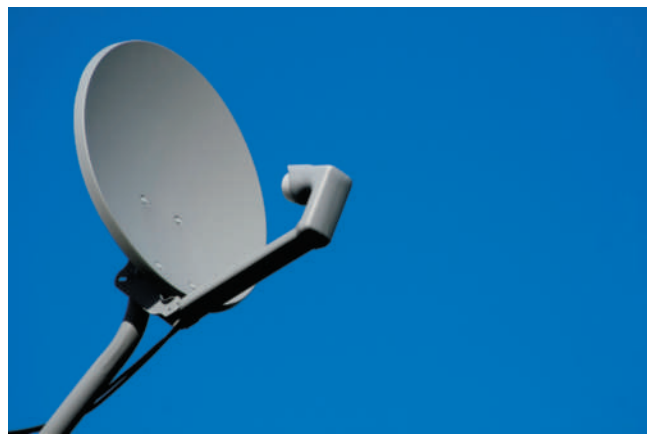
FIGURE 25-5 (A) A digital satellite system receiver, and a remote control. (B) An 18 in. (450 mm) dish-type satellite antenna.
