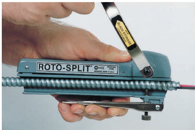
FIGURE 4-26 This is an example of a tool that precisely cuts the outer armor of armored cable, making it easy to remove the armor with a few turns of the handle.
