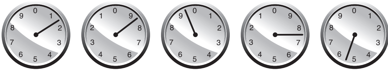
FIGURE 29-5 One month later, the meter reads 18,975 kilowatt-hours, indicating that 303 kilowatt-hours were used during the month.
