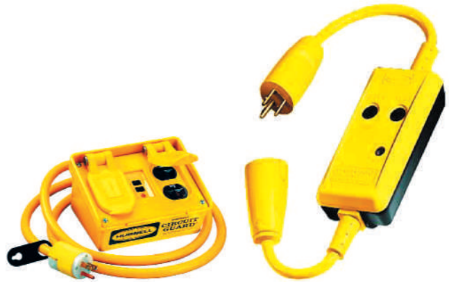
FIGURE 6-25 Cord-and-plug-connected portable GFCI devices are easy to carry around. They can be used anywhere when working with electrical tools and extension cords. These devices operate independently and are not dependent on whether the branch circuit is GFCI protected. These portable GFCI in-line cords are relatively inexpensive and should always be used when using portable electric tools.
