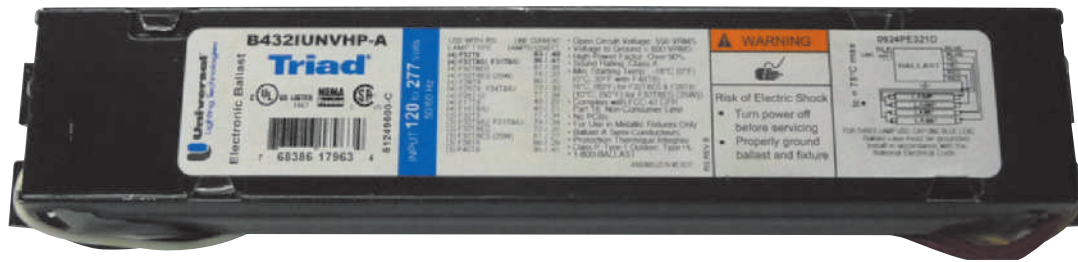
FIGURE 7-13 An electronic Class P ballast, thermally protected as required in 410.130(E) . Electronic ballasts provide improved performance in fluorescent lighting installations. Electronic ballast lighting systems are 25% to 40% more energy efficient than conventional magnetic (core and coil) ballast fluorescent systems.
