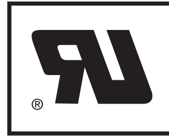
FIGURE 1-10 The recognized components mark.
