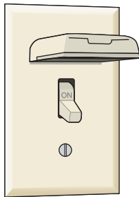
FIGURE 5-9 Switch is protected by a weatherproof cover.
