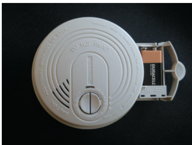
FIGURE 26-3 An ac-dc smoke alarm that operates on 120 volts ac as the primary source of power and a 9-volt battery as the secondary source of power. In the event of a power outage, the alarm continues to operate on the battery.
