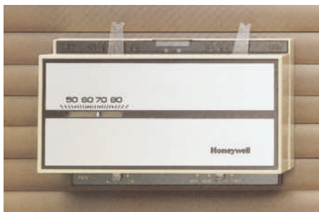
FIGURE 23-2 Thermostats for electric heating systems. A thermostat or other switching device that is marked with an OFF position must open all ungrounded conductors of the circuit when turned to the OFF position. Typical mounting height is 52 in. (1.3 m) to center.
