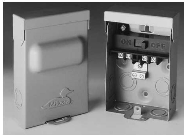
FIGURE 23-21 (A) is a pull-out fusible disconnect. Fuses are inserted into fuse clips on the pull-out device. Insert the pull-out device for ON, and remove the pull-out device for OFF. (B) is a nonfusible disconnect, available in 30- and 60-ampere ratings at 240 volts. Both have padlock provisions to prevent unauthorized tampering. Air-conditioner disconnects are available that have a GFCI receptacle as part of the disconnect enclosure. The GFCI receptacle must be wired to a separate 20-ampere, 120-volt branch circuit.
