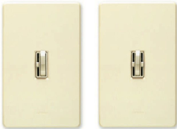
FIGURE 9-13 Two types of fan/light controls. One has a toggle switch for turning a ceiling fan off and on, plus a “slider” that provides 3-speed control of the fan. The other has a toggle switch for turning a light off and on, plus two “sliders,” one for 3-speed control of a ceiling fan and the other for full range dimming of lighting.
