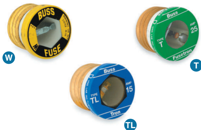
FIGURE 28-7 Three types of plug fuses: single-element, nontime-delay (W); dual-element, time-delay (T); loaded link, time-delay (TL).
