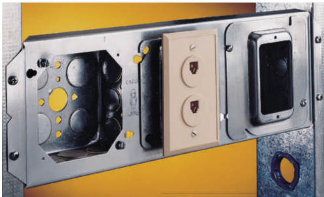
FIGURE 2-25 A bracket for use on steel framing members. The bracket spans the space between two studs. Note that more than one box can be mounted on this bracket.
