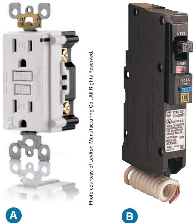
FIGURE 6-7 (A) A ground-fault circuit interrupter and tamper-resistant receptacle, and (B) a ground-fault circuit interrupter circuit breaker. The switching mechanism of a GFCI receptacle opens both the ungrounded “hot” conductor and the grounded conductor. The switching mechanism of a GFCI circuit breaker opens the ungrounded “hot” conductor only.
