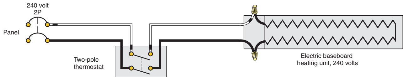
FIGURE 23-4 Wiring for a single electric baseboard heating unit. The thermostat is a line-voltage thermostat. See Figure 23-3 caption for color-coding requirements.
