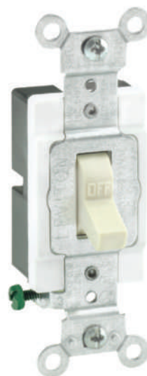
FIGURE 5-32 Single-pole toggle switch. Note that this switch has a terminal for the connection of an equipment ground conductor. Thus, when a metal face plate is installed, it will be grounded. See 404.9(A) and (B).
