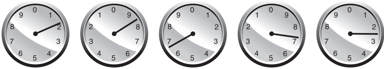
FIGURE 29-4 The reading of this five-dial meter is 18,672 kilowatt-hour.
