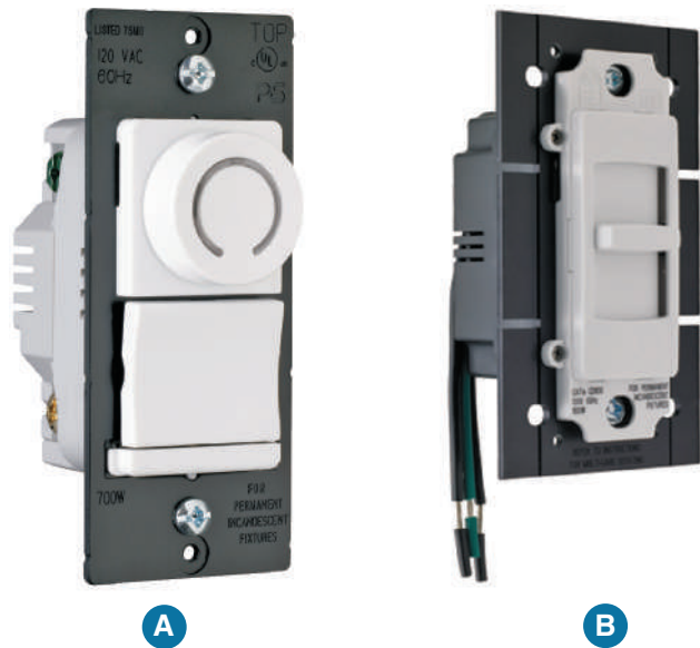
FIGURE 13-10 Some typical electronic dimmers. Both perform the same function of varying the voltage to the connected incandescent lamp load: (A) rotating knob; (B) slider knob.
