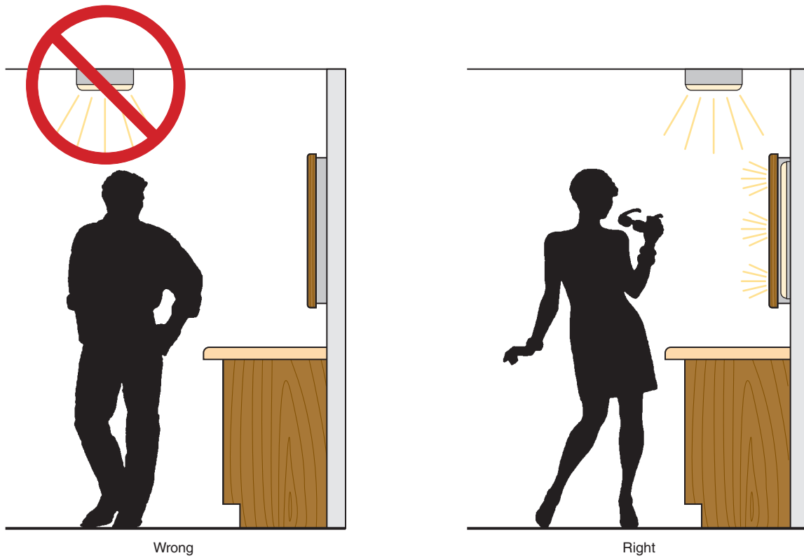
FIGURE 10-5 Positioning of bathroom luminaires. Note the wrong way and the right way to achieve proper lighting.
