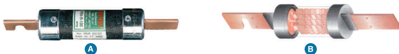
FIGURE 28-8 Cartridge-type dual-element fuse (A) is a 250-volt, 100-ampere fuse. The cutaway view in (B) shows the internal parts of the fuse. When this type of fuse has a rejection slot in the blades of 70–600-ampere sizes, or a rejection ring in the end ferrules of the 0–60-ampere sizes, it is a UL Class RK1 or RK5 fuse.
