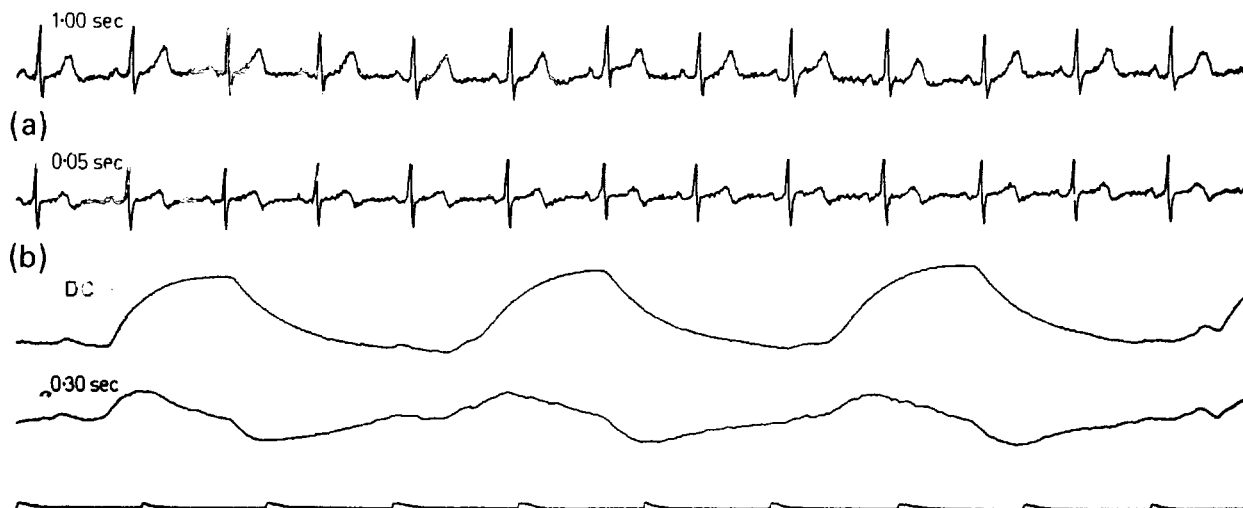
Figure 10.6—(a) Recording of ECG from electrodes on upper arms with time constants of 1 s and 0.05 s respectively. (b) Recording of respiration from thermistor in nostril with time constants of infinity (d.c. setting) and 0.3 s respectively
