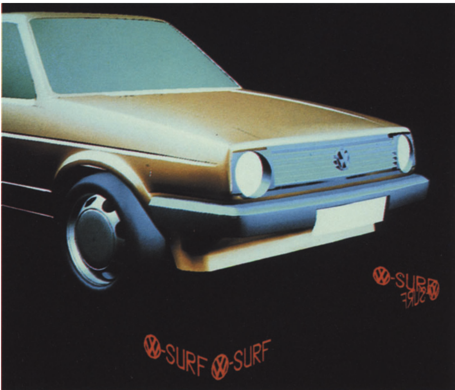
Fig. 8.7. Shaded picture representation of the front portion of a car (courtesy of Volkswagenwerk, Wolfsburg)
