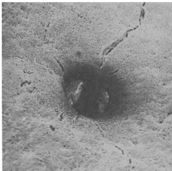
Fig. 1 Crater produced by pulse irradiation on NC, enlarged 1000x .
