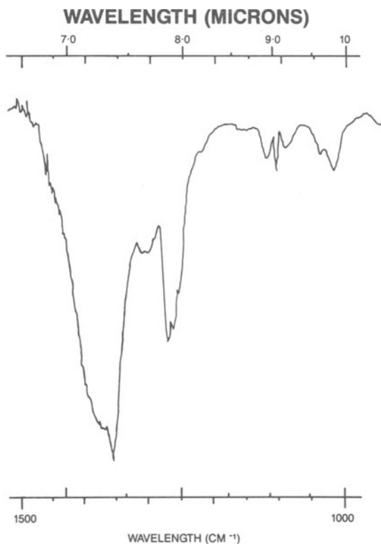
Figure 5. IR spectra of gaseous products formed from \text{CO}_2 laser multiphoton decomposition of RDX.
