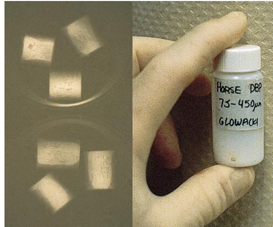
Fig. S28F: Decalcification typically takes 5–9 days; periodic radiographic exposures monitor progress. When decalcification is complete, the bone pieces are frozen in individual sterile vials.
