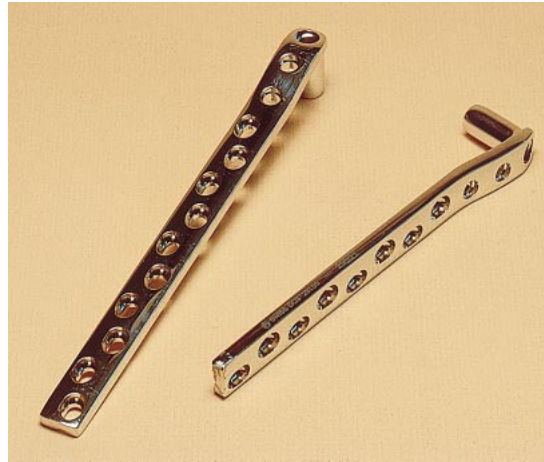
Fig. S14B: Two DCS plates of different lengths are depicted, demonstrating their configuration. The plates are manufactured from 316 L stainless steel. The cross-section measures 16 x 5.8 mm. The two holes next to the barrel are round and allow insertion of 6.5 mm cancellous bone screws.
