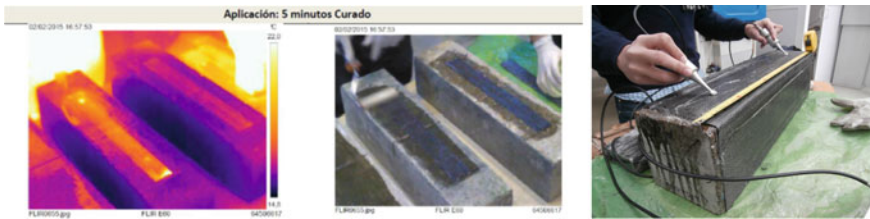
Fig. 1 Non-destructive testing of infrared thermography and ultrasound performed
