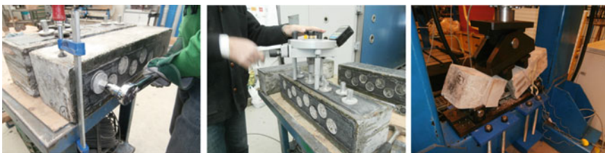
Fig. 2 Pull off and Shear torsion destructive testing
