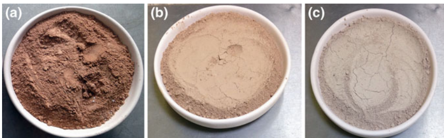
Fig. 2 RMF dehydrated at 800 ^{\circ}\text{C} samples: a concrete waste family, b mortar waste family, c adhesive mortar waste
