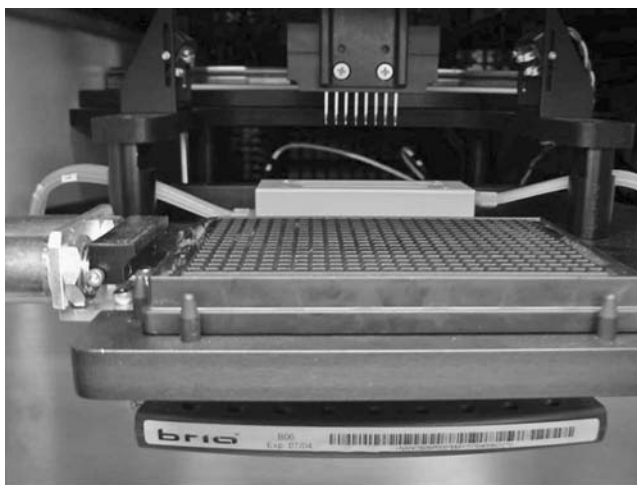
FIGURE 6.8 Autosampler employed in \mu PLC system. Note eight-head autosampler above the rinsing station.
