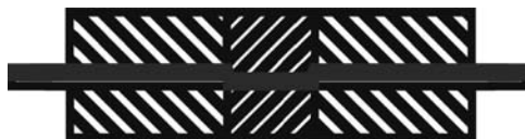
FIGURE 6.9 Individual flow cell employed for UV absorbance detection in \mu PLC systems. The shaded channels represent fluid (sample + mobile phase) pathways; the clear channels represent the light pathways. The flow cell counts with a U-shape design since liquid is transported in a U-shape within the flow cell.
