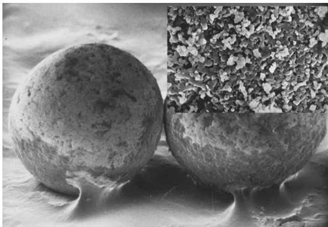
FIGURE 13.8 Scanning electron micrograph showing nonreticulated porous structures of standard spherical silica particles.
