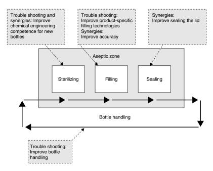
*Figure 4.13* Trouble shooting and technological synergies at the Aseptofill filling machine
