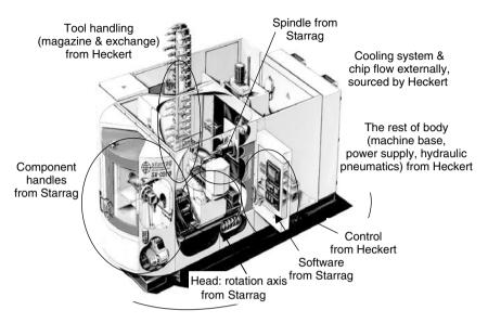
Figure 4.35 SX-051, Platform 3 developed on Heckert's base machine
