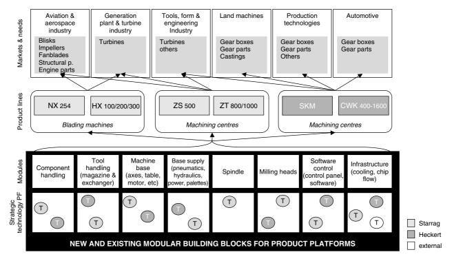
Figure 4.38 Modular building blocks for Starrag and Heckert product platforms
