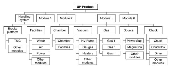
*Figure 4.28* Modular structure of a Unified Platform product
