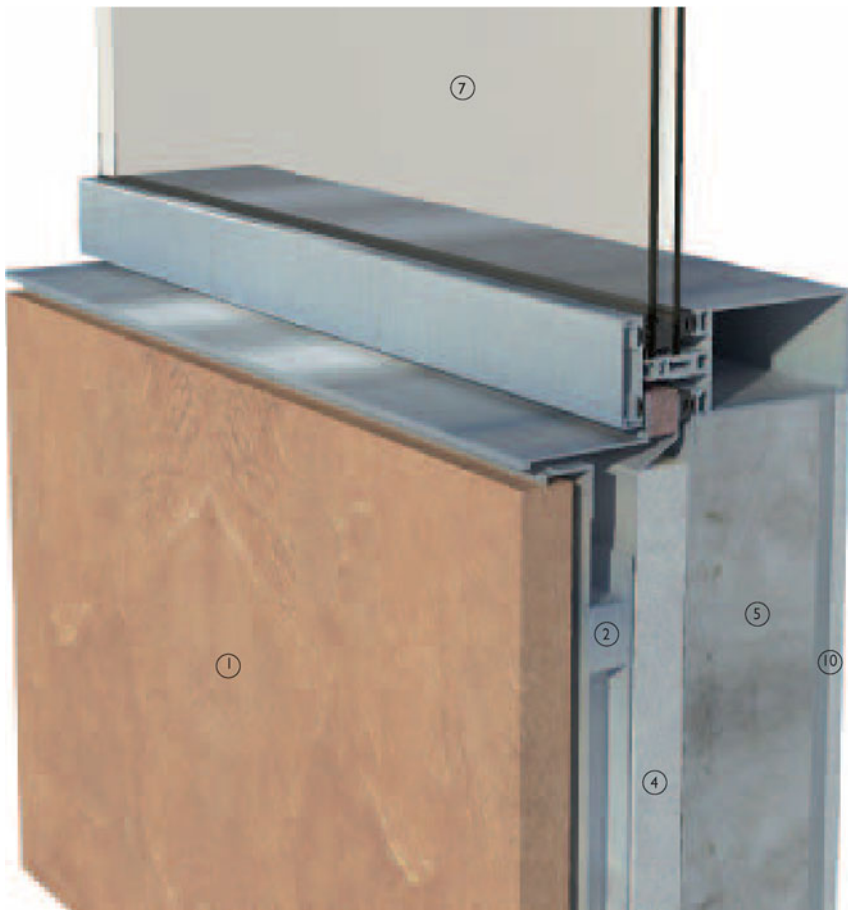
3-D view of bottom of window opening in terracotta rainscreen facade
