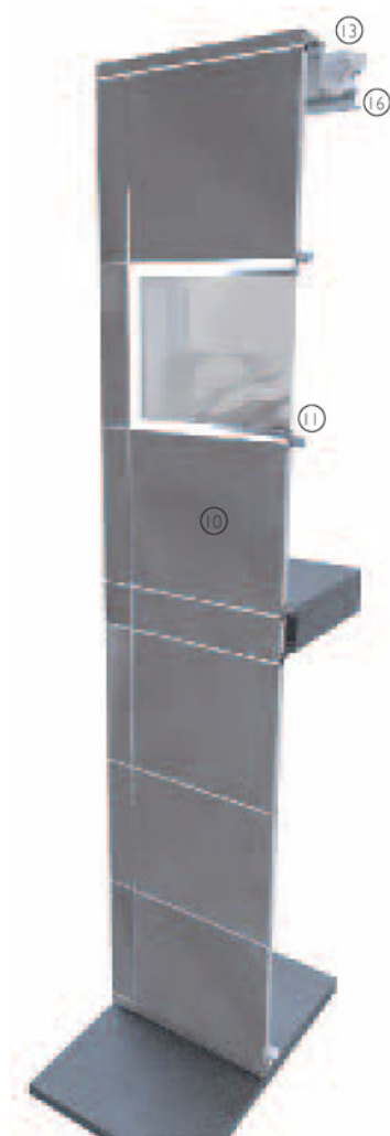
3-D view of composite panel facade assembly with flush glazing and concealed parapet
