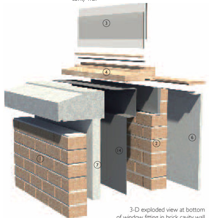
3-D view at bottom of window opening in brick cavity wall
