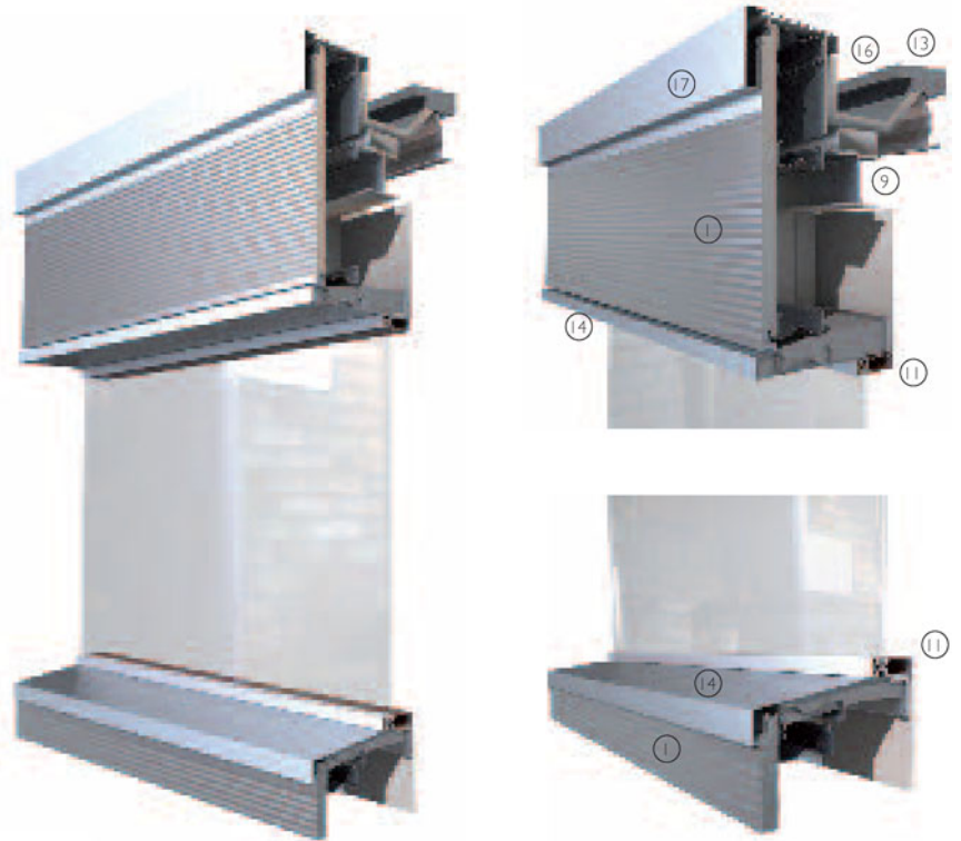
views of composite panel curtain wall with recessed window with deep metal reveal, with cill and gutter detail
