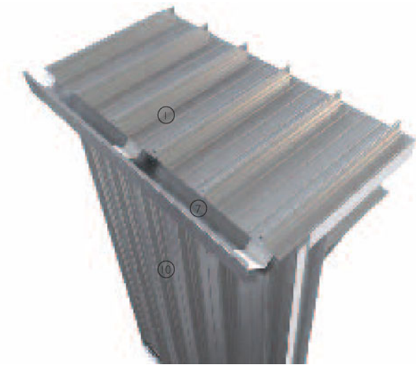
3-D view of flat profiled metal sheet roof construction
