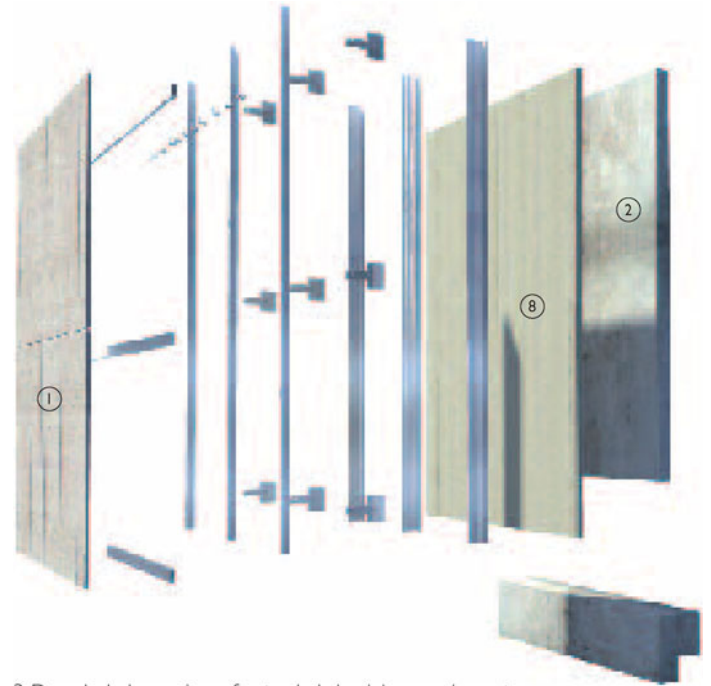
3-D exploded overview of extruded aluminium carrier system
