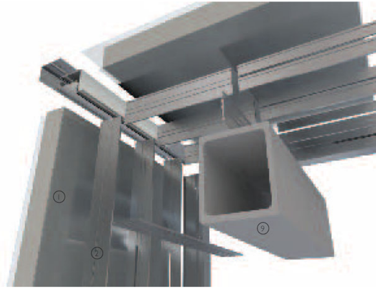
3-D exploded view of small rooflight
