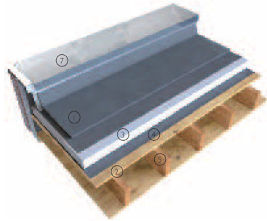
3-D view of typical flat timber roof construction with rigid insulation above roof structure
