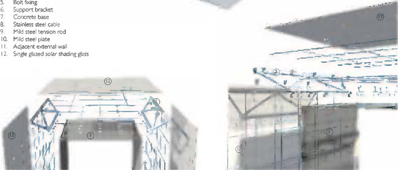
3-D exploded views showing twin wall roof with double glazed units, steel truss support system and glazed solar shading assembly
