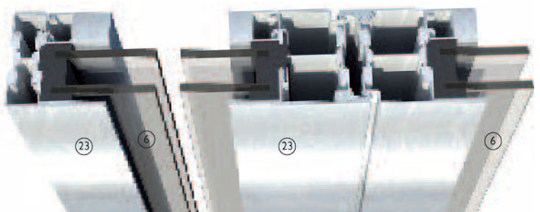
3-D view of outward opening pressed steel door with thermal break
