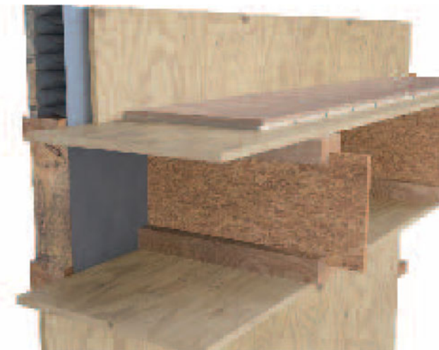
3-D view of floor to wall junction
