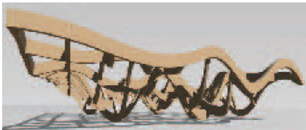
Panelisation of geometry for manufacture.
