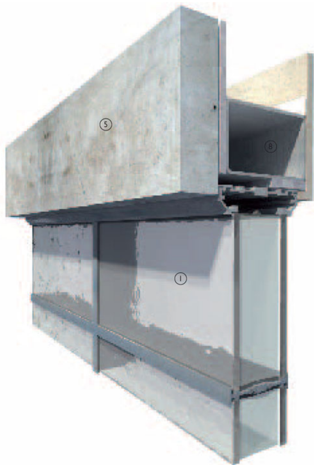
3-D view of glass block window supported on thermally broken aluminium framework
