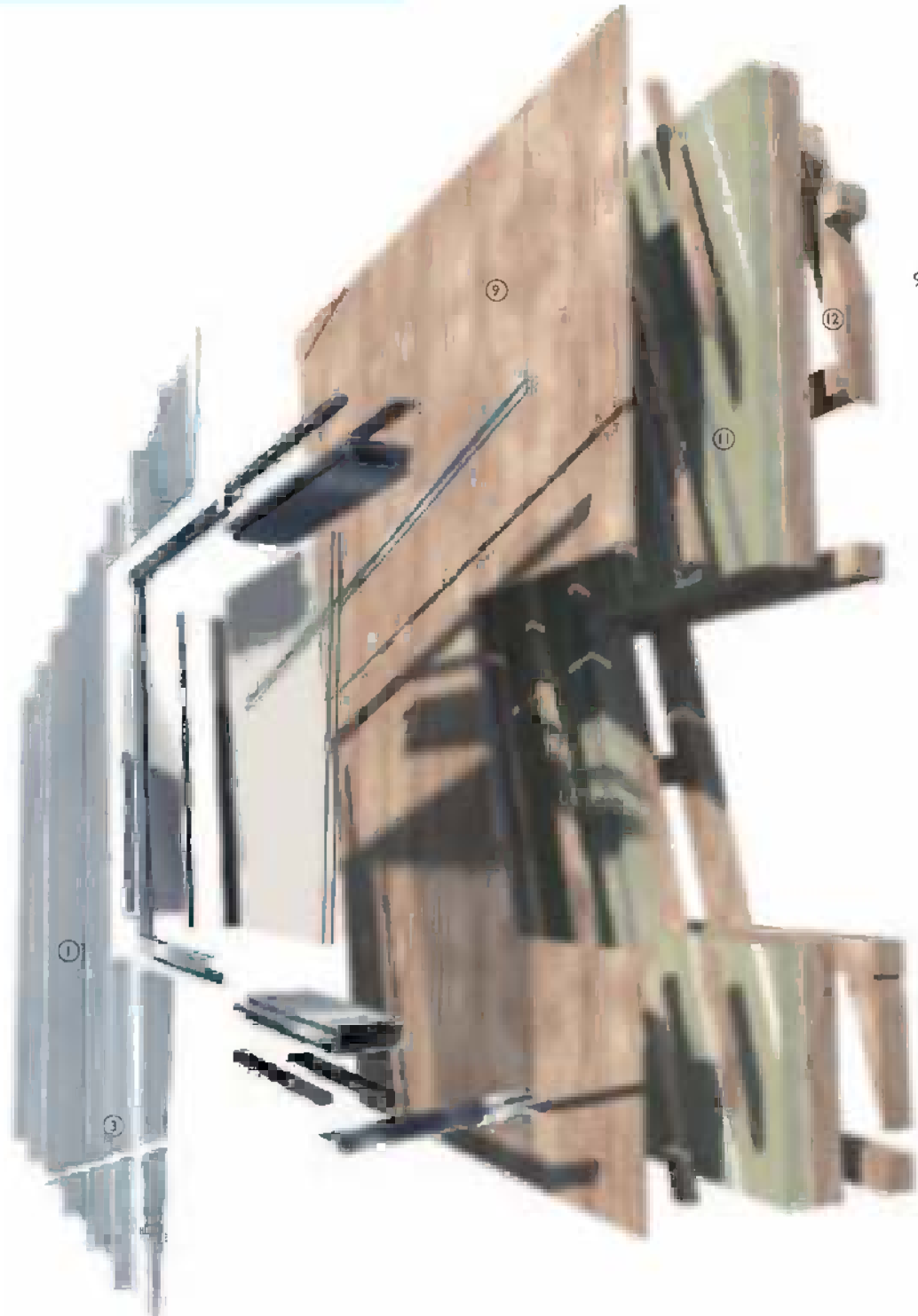
3-D exploded view of horizontally set folded metal sheet facade with angled seam lines
