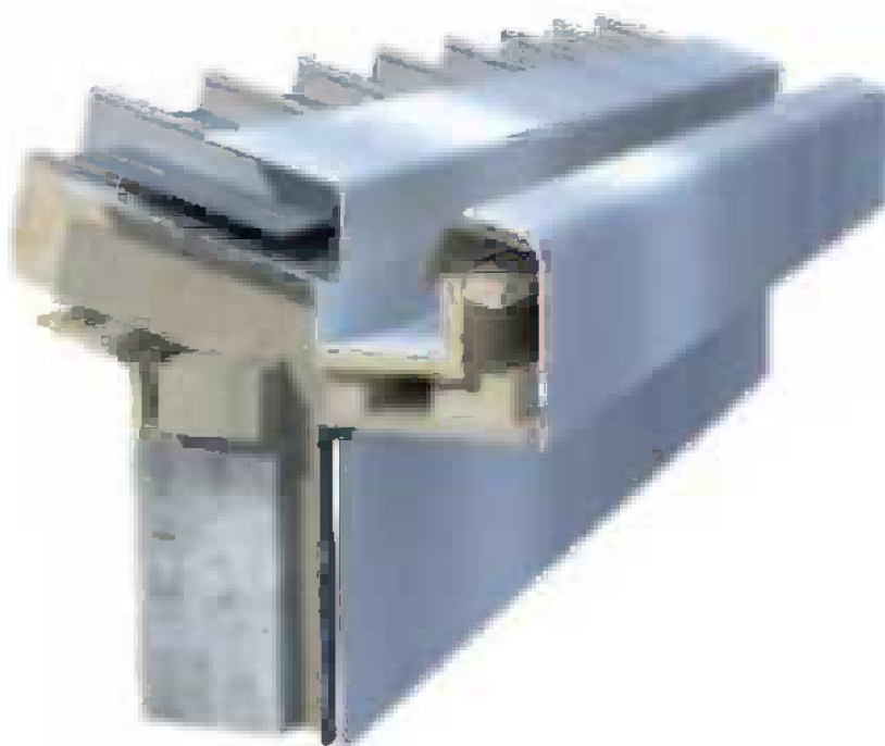
3-D views showing eaves and gutter condition
