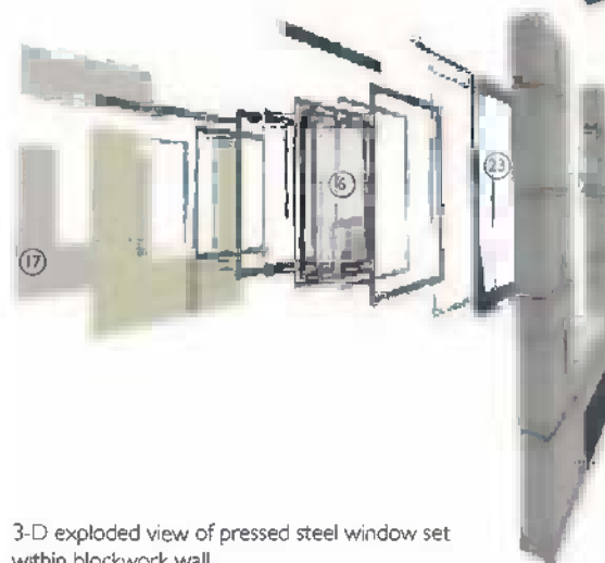
3-D view of pressed steel window detail in masonry cavity wall construction
