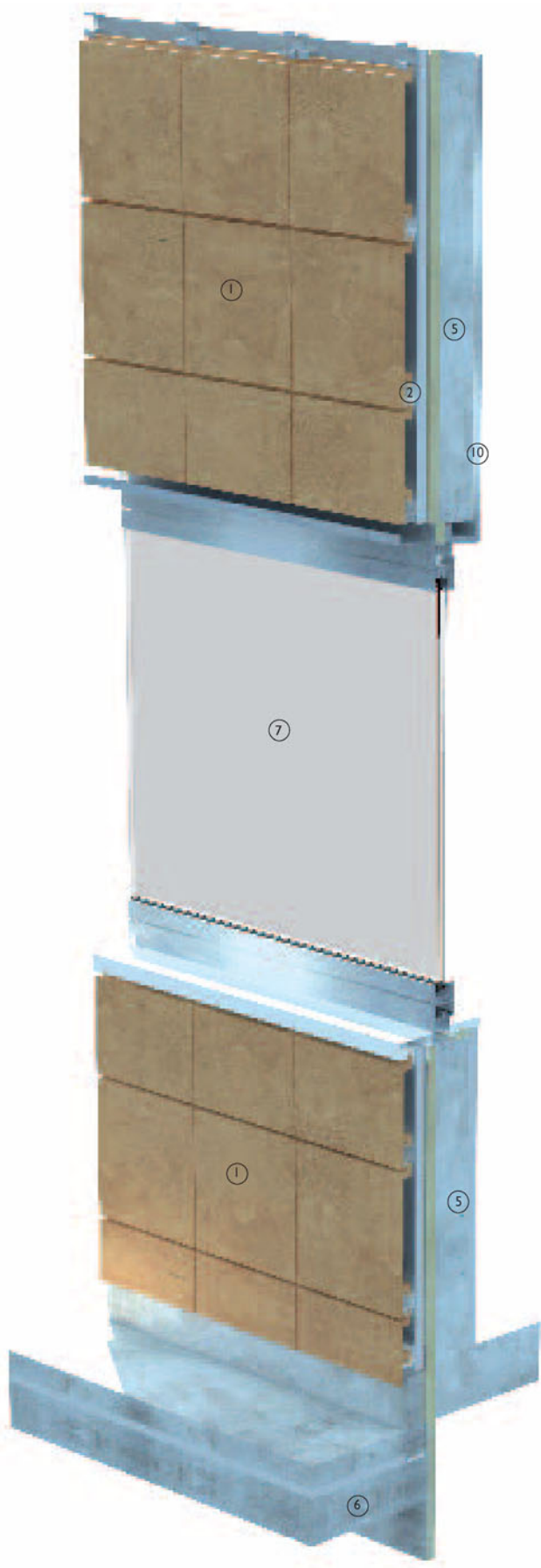
3-D view of terracotta rainscreen assembly, hung from individual aluminium clips and horizontally-set support rails
