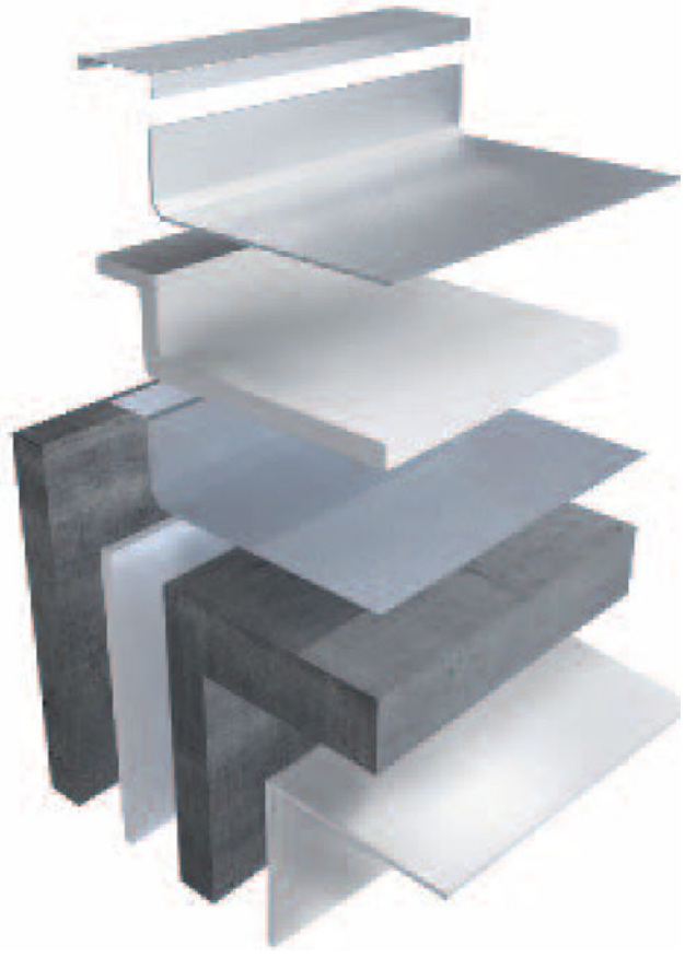
3-D exploded loadbearing concrete wall gutter detail
