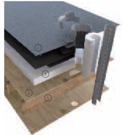
3-D exploded view of flat roof with a bitumen-based sheet membrane, with pipe penetration
