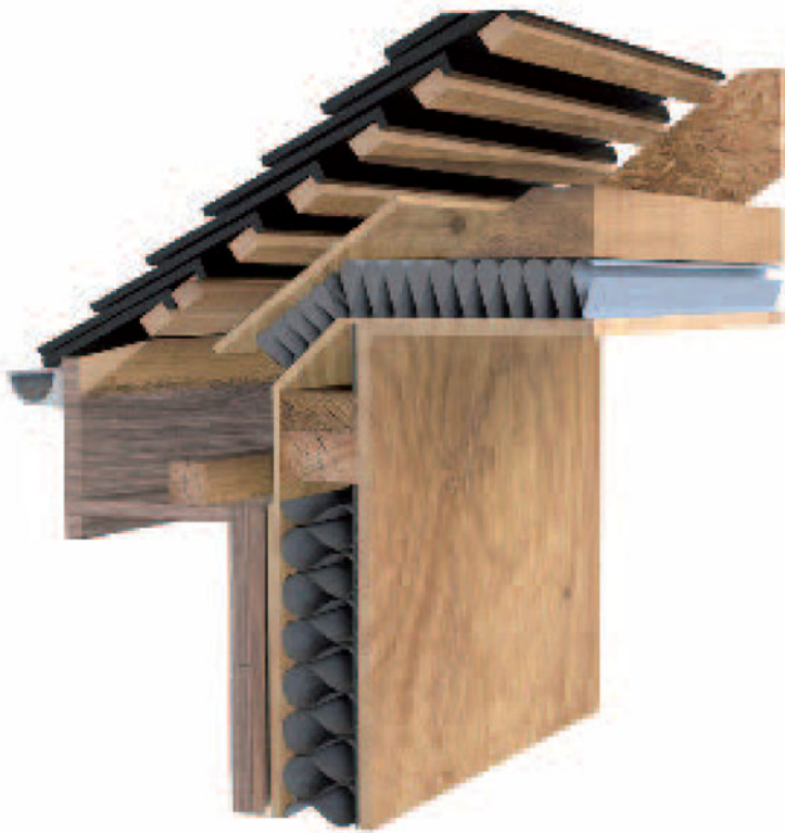
3-D view of eaves condition
