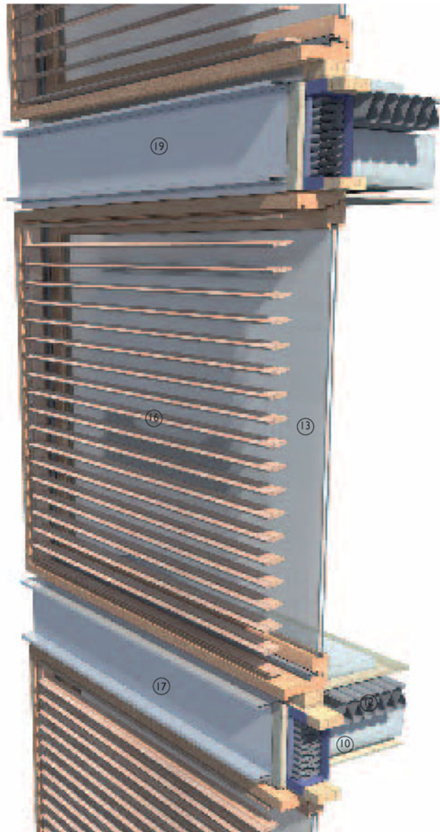
3-D views showing connection between timber cladding panel and supporting frame
