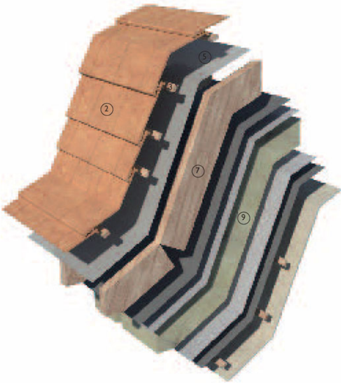
3D exploded view showing internal fold on roof using interlocking tiles
