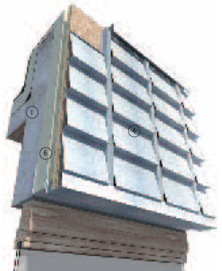
3-D views showing recessed timber window opening in metal rainscreen shingle cladding system
