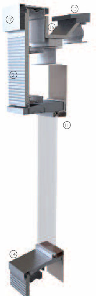
3-D section of composite panel curtain type wall with recessed window with deep metal reveal
