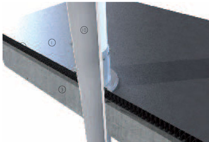
3-D view of bonded method. Pipe penetration
