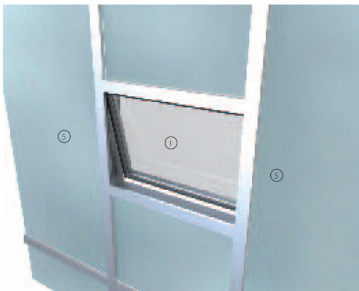
3-D view of top hung aluminium window
