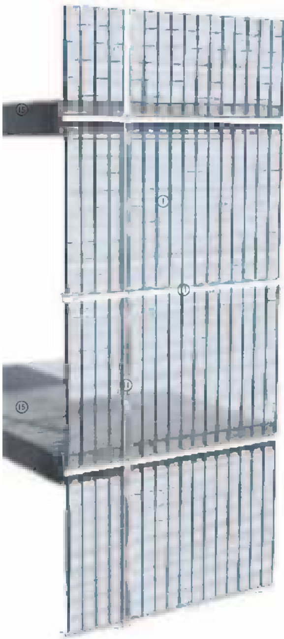
Vertical section & elevation 1:25. Glass block wall supported from steel frame
