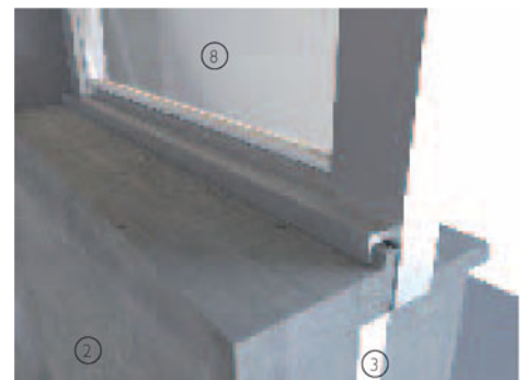
3D detail view of precast concrete wall
