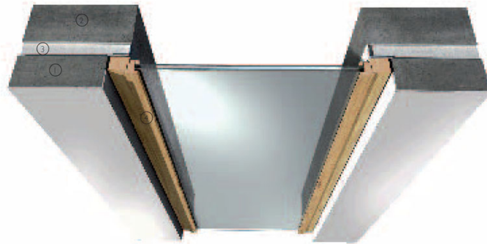
3-D view of window in an in-situ cast concrete wall cast in two skins with rigid closed cell insulation between skin
