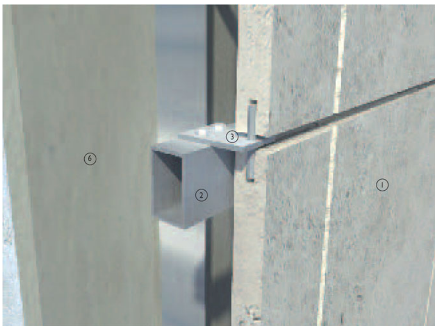
3-D view of stainless fixing method for extruded aluminium carrier system
