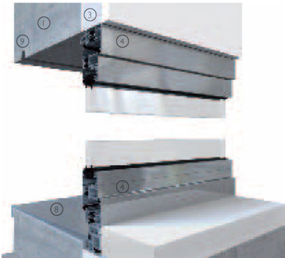
3-D view of window junction in an in-situ concrete wall cast as a monolithic construction with internal thermal insulation
