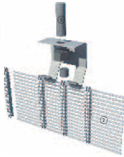
3-D exploded view of hooked metal mesh fixing
