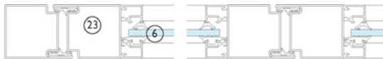
Horizontal section 1:10. Inward opening pressed steel single glazed fire resisting doors without thermal breaks
