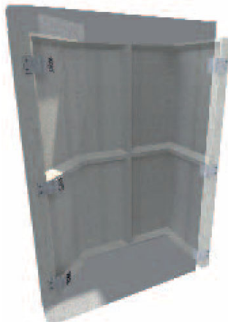
3-D view of wall clad with small GRC panels
