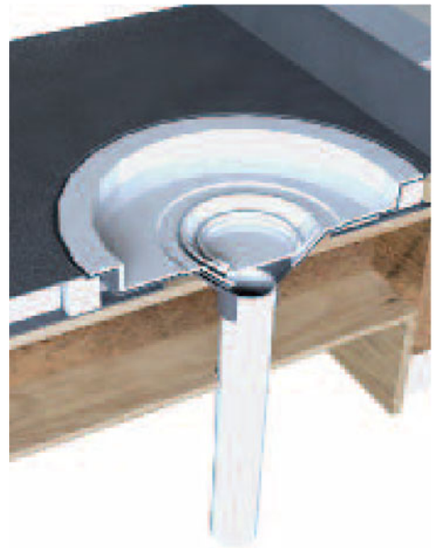
3-D view of flat roof with a bitumen-based sheet membrane, drain outlet detail
