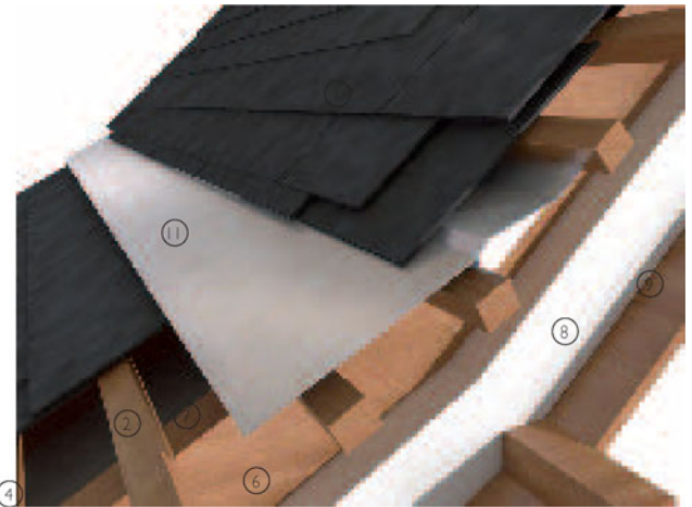
3-D view of internal fold detail in timber pitched roof construction with roofing slates
