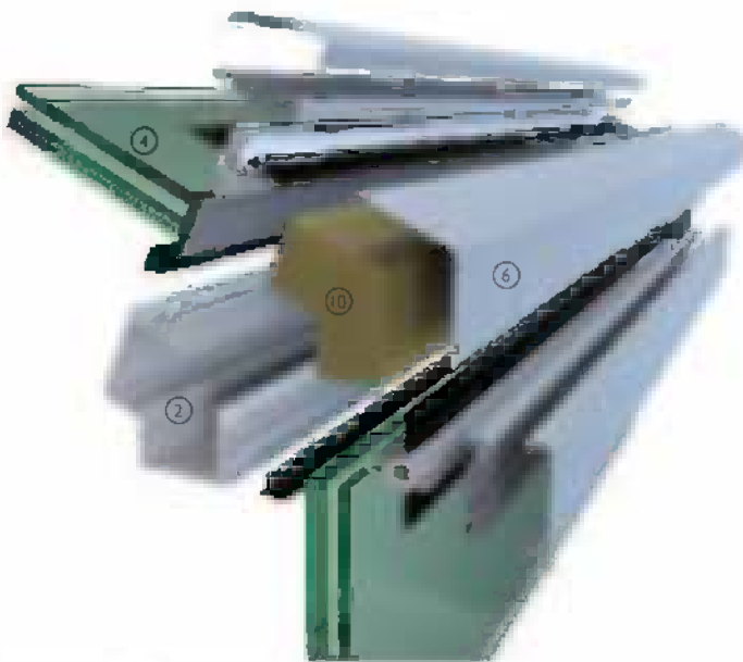
3-D exploded view of greenhouse eaves detail
