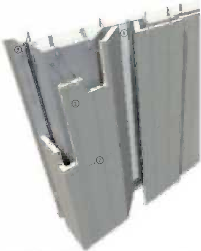
Cutaway 3-D view of wall clad in precast concrete cladding panels, showing wall construction
