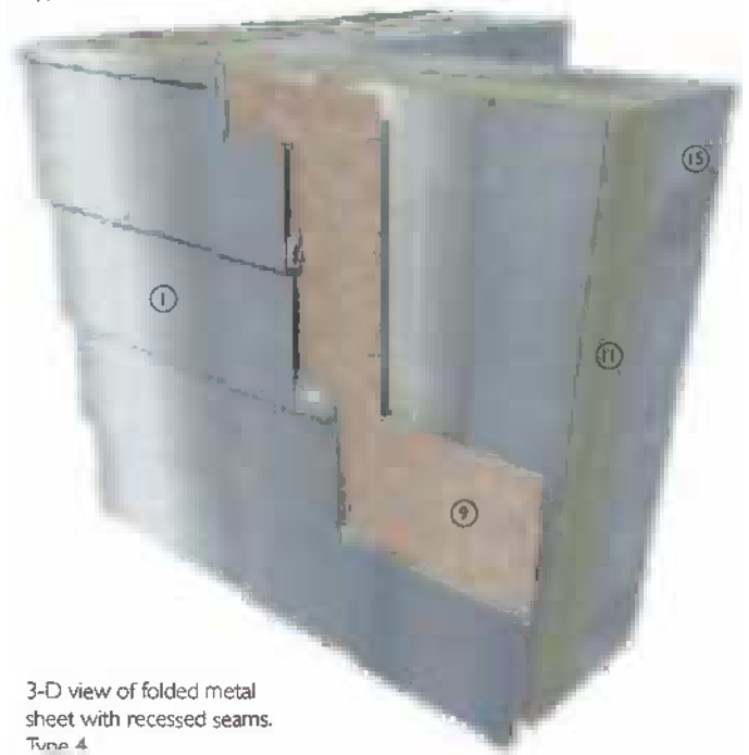
3-D view of folded metal sheet with recessed seams. Type 4
