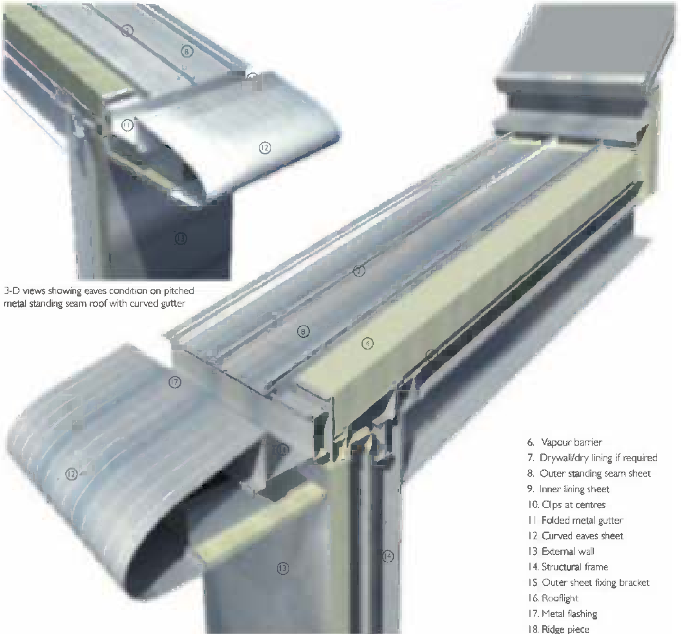
Vertical section 1:10. Eaves with curved gutter.
