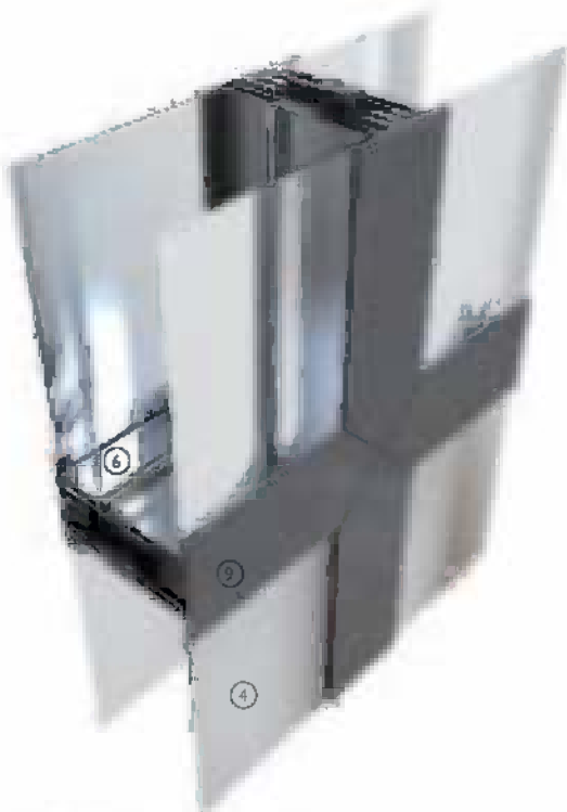
3-D detailed view of panel junction
