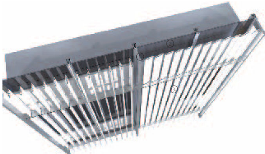
3-D view of frame supported metal louvres used as a shading device in front of glazed curtain wall
