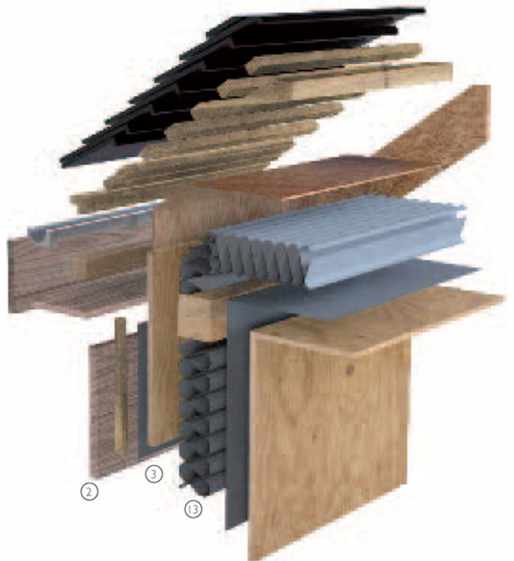
3-D exploded view of eaves condition
