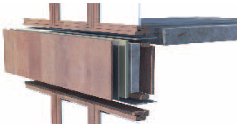
3-D exploded detail view of storey-height timber window construction at upper floor level
