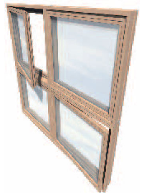
3-D view showing side hung window
