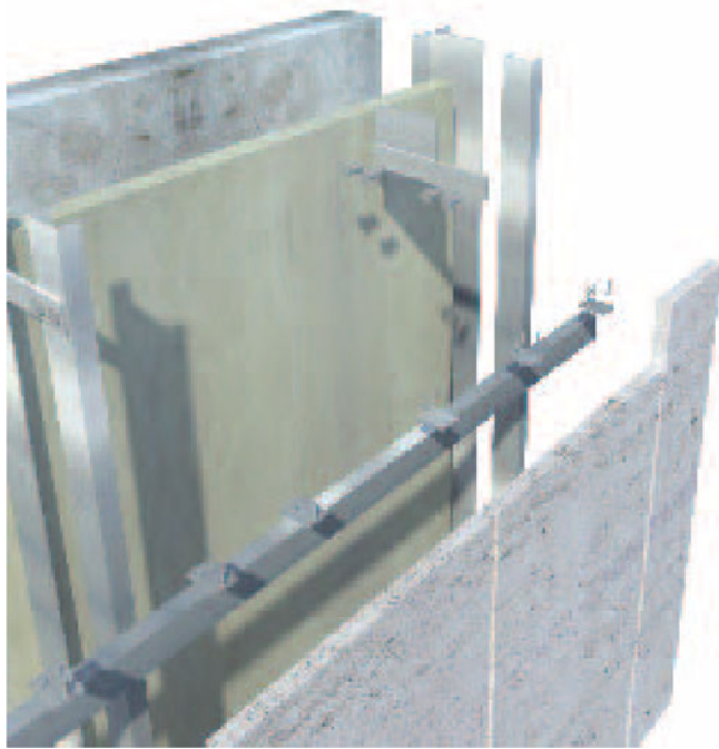
3-D exploded detail view of extruded aluminium carrier system
