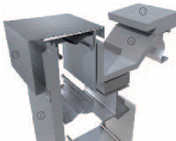
3-D view of gutter detail
