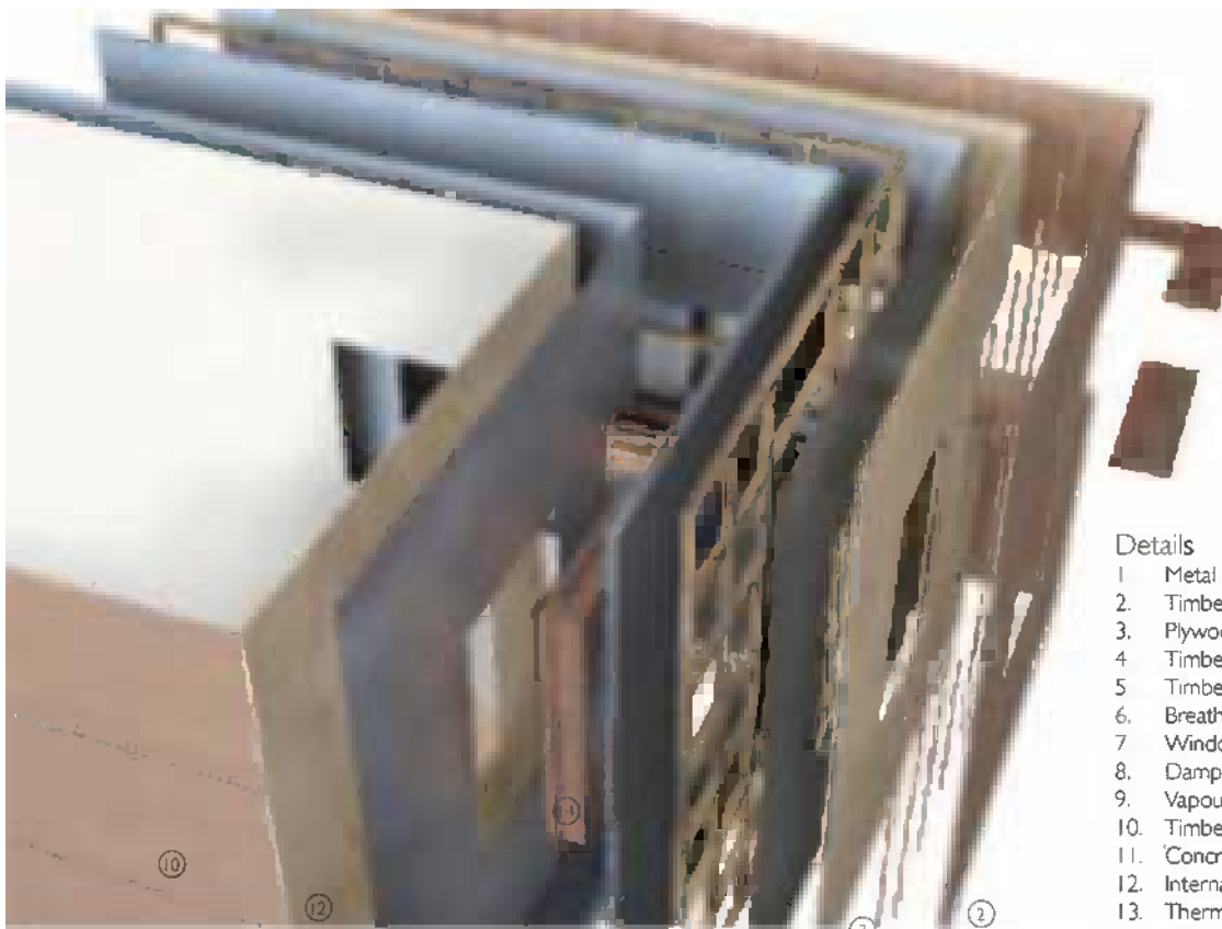
3-D exploded view of timber framed wall with two openings
