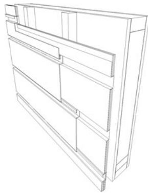
3-D view of folded metal sheet with recessed seams
