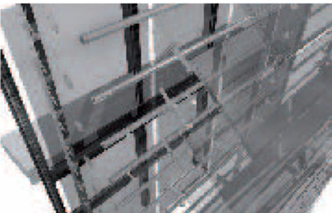
3-D detailed views of frame supported solar control glass louvres used as a shading device in front of glazed curtain wall
