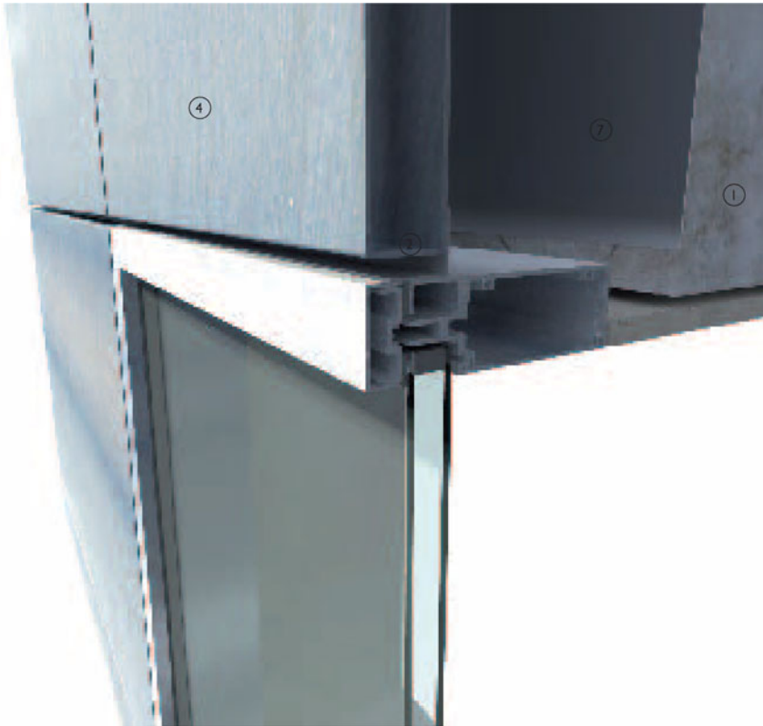
3-D view of curtain wall type glazing set flush with metal rainscreen cladding. Type 3
