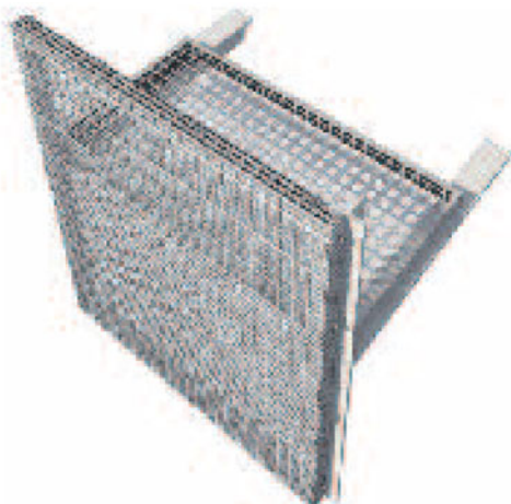
3-D view of metal mesh fixed to steel frame with maintenance deck behind
