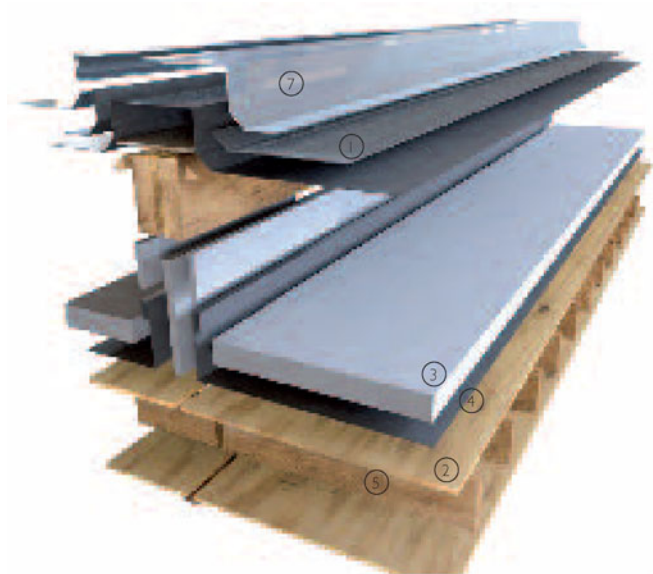
3-D exploded view of expansion joint in a flat roof with a bitumen-based sheet membrane
