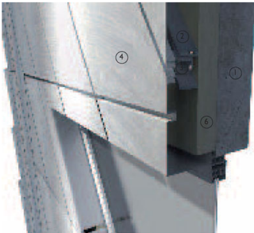
Horizontal section 1:10. Internal corner connection between metal rainscreen panels with open horizontal joints and interlocking vertical joints
