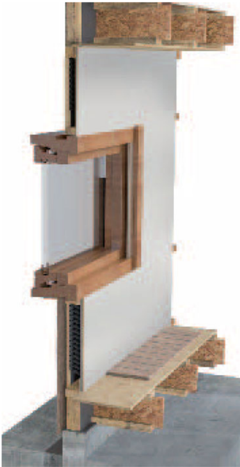
3-D view of timber wall construction
