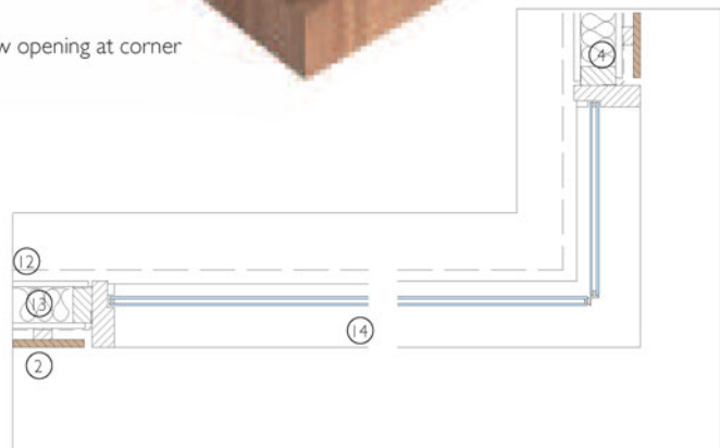
Horizontal section 1:25. Window opening at corner
