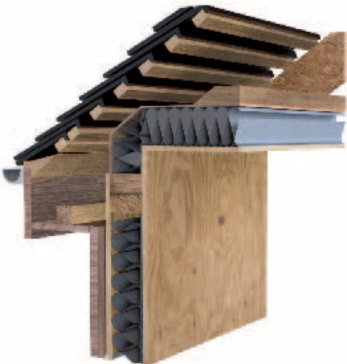
3-D view of eaves condition
