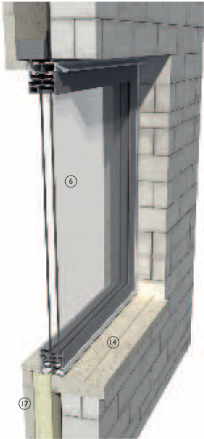
3-D view of double glazed steel frame window set in cavity wall construction
