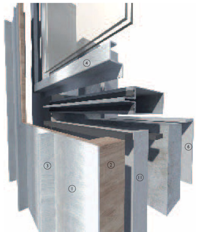
3-D exploded view of window opening in horizontally set folded metal sheet facade with vertical seam lines
