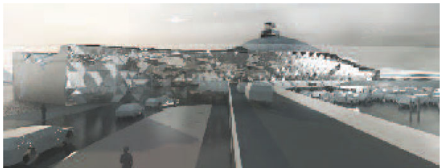
Envelope option of hexagonal unitised panels based on triangular units set into them.
