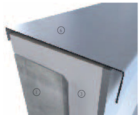
3-D view of metal flashing on in-situ cast concrete wall cast in two skins with rigid closed cell insulation between skins
