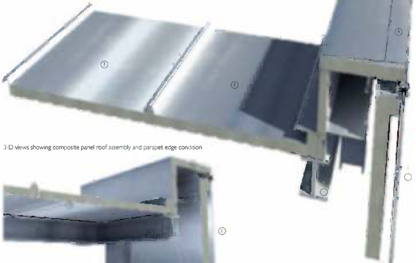
3-D view of verge with parapet upstand
