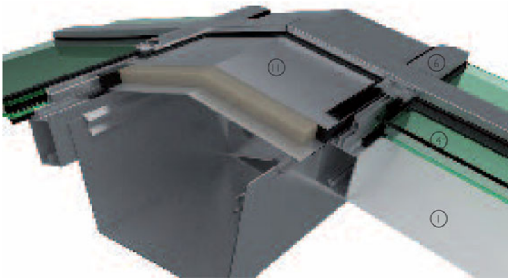
3-D view of capped glazing ridge detail
