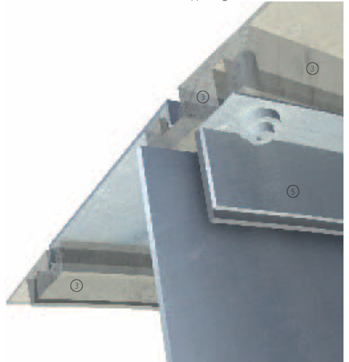
3-D view showing fixing method for GRP roof panel formed with steel structure
