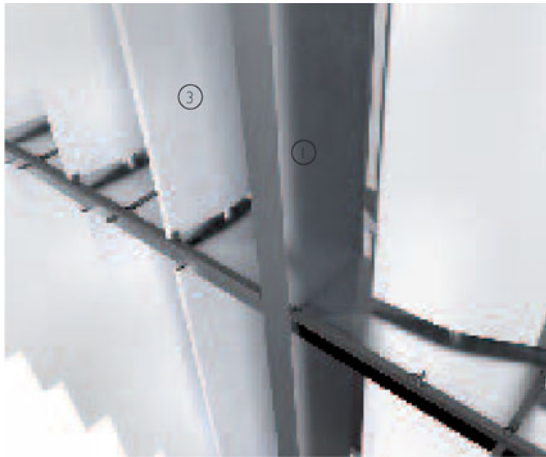
3-D detail view of metal louvres
