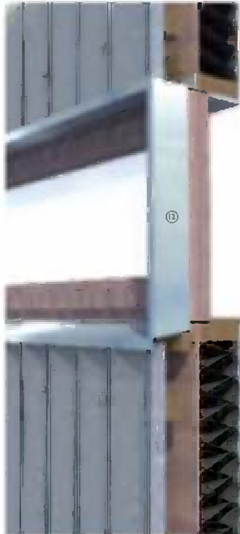
3-D section detail of polycarbonate rainscreen
