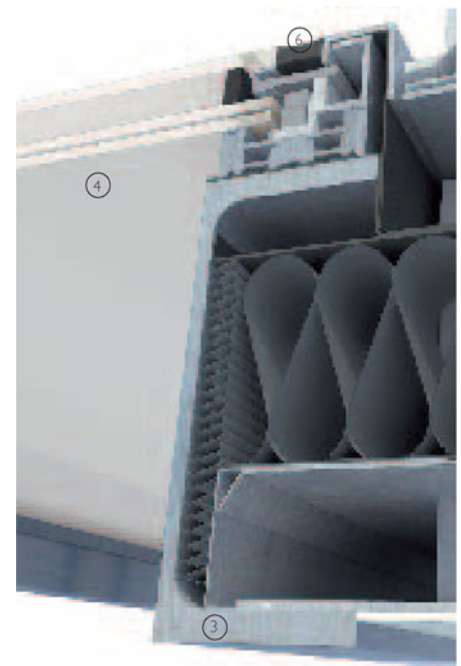
3-D view showing window-wall junction
