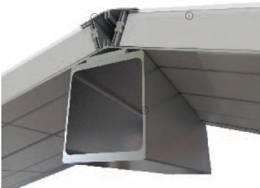
Vertical section 1:5. Large rooflight eaves
