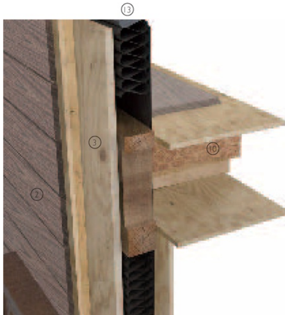
3-D view of floor to wall junction
