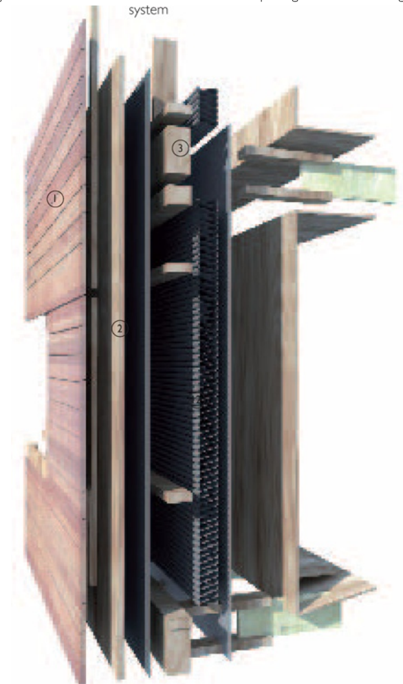
3-D exploded view of timber cladding panel wall assembly
