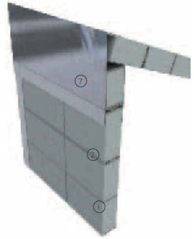
3-D view of large rooflight monopitch ridge
