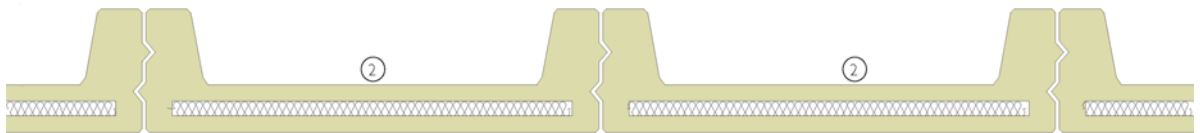
Horizontal section 1:25. Joint between precast concrete panels
