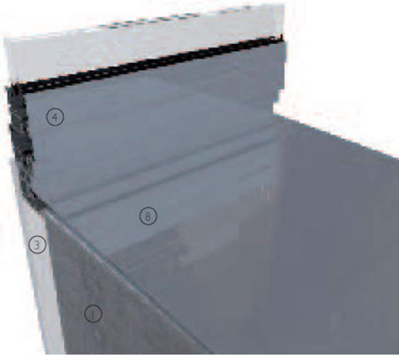
3-D view of window and external cill
