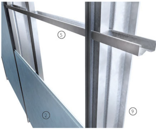
3-D view of framework supporting composite panels interlocking horizontally with vertical capping piece
