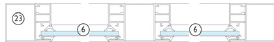
Horizontal section 1:10. Fixed pressed steel single glazed fire resisting doors without thermal breaks
