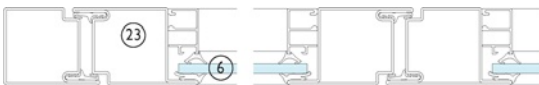
Horizontal section 1:10. Outward opening pressed steel single glazed fire resisting doors without thermal breaks
