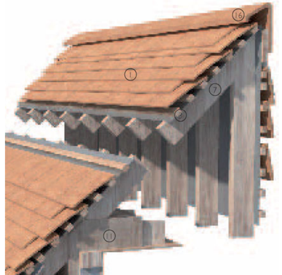
3-D view of plain tiles on monopitch roof
