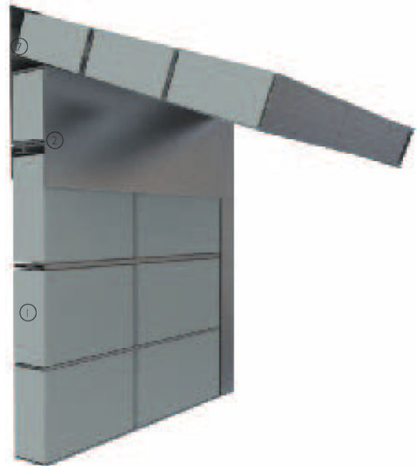
3-D view of large rooflight monopitch ridge
