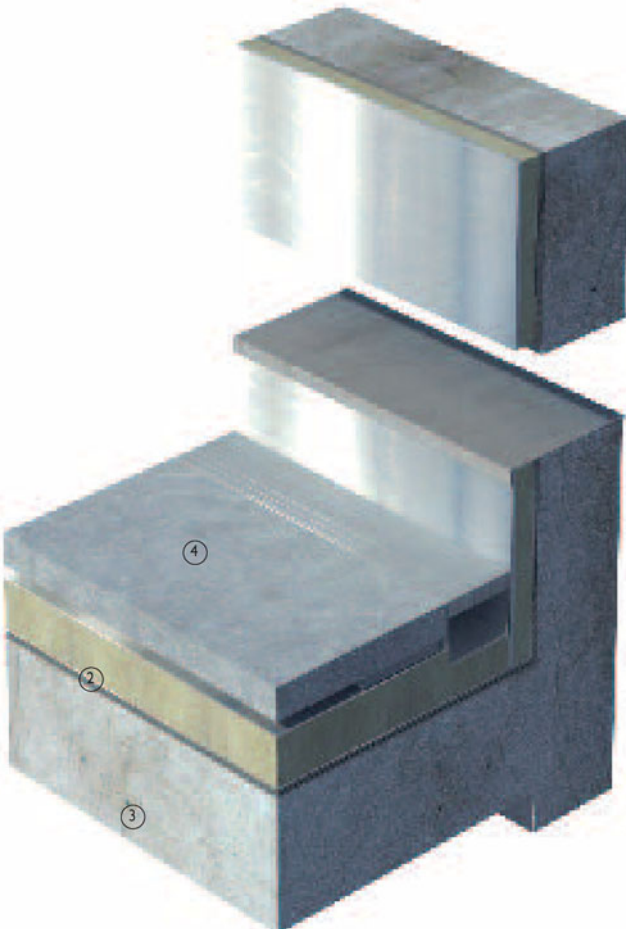
3-D section view showing junction of external wall and roof with overflow
