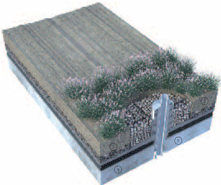
3-D details of pipe penetration in heavily planted roof
