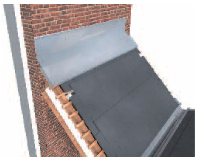
3-D view of abutment detail of timber pitched roof construction with roofing slates
