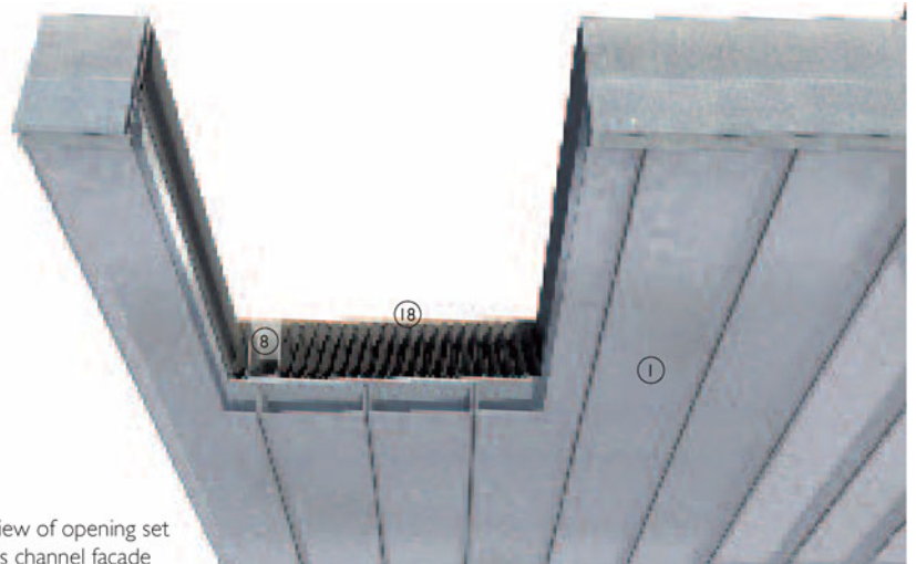
Vertical section 1:10. Interlocking horizontally set glass channels used as window
