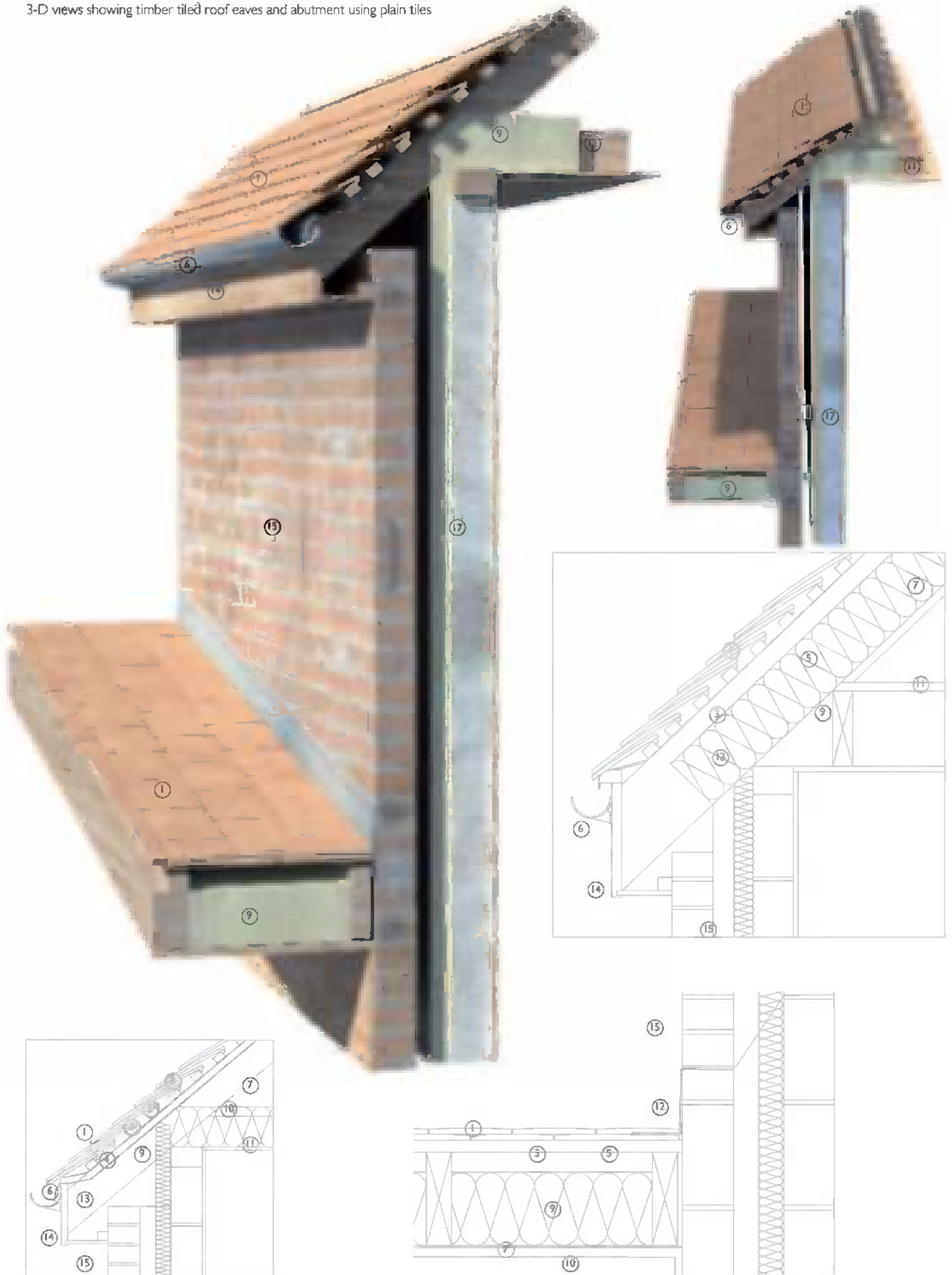
Vertical section I 20. Plain tiles. Eaves
