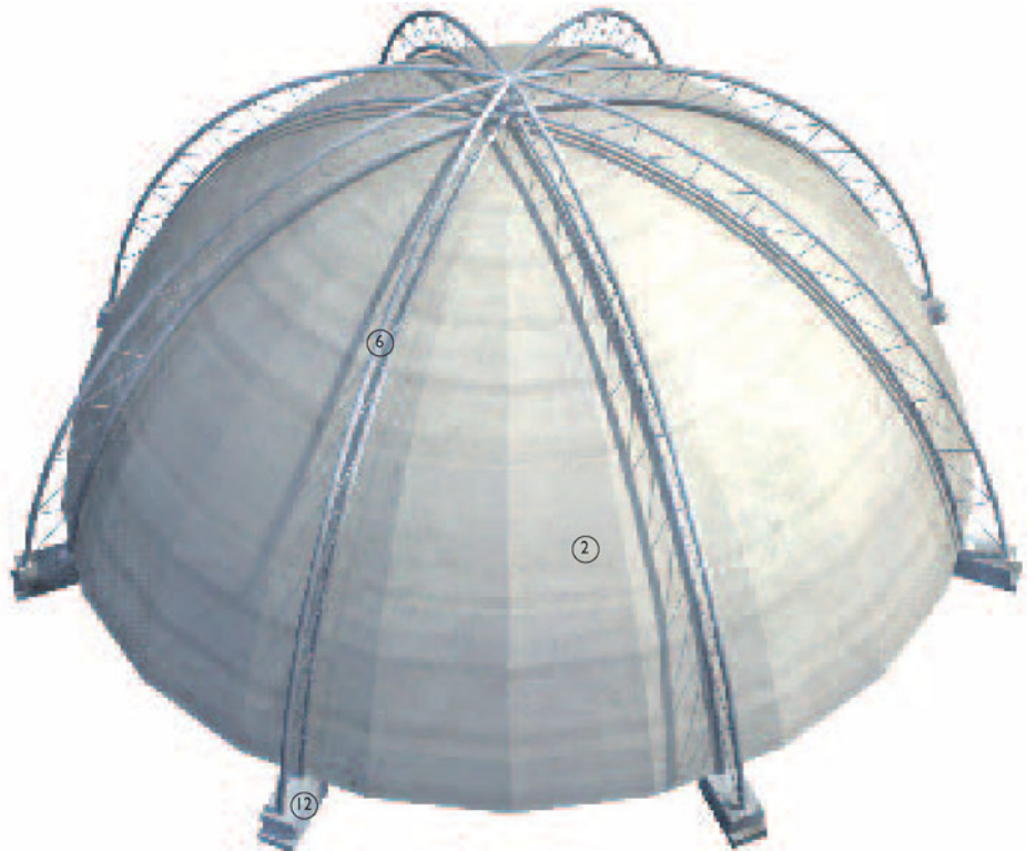
3-D view showing hemispherical dome formed with GRP shell panels and external steel structural truss
