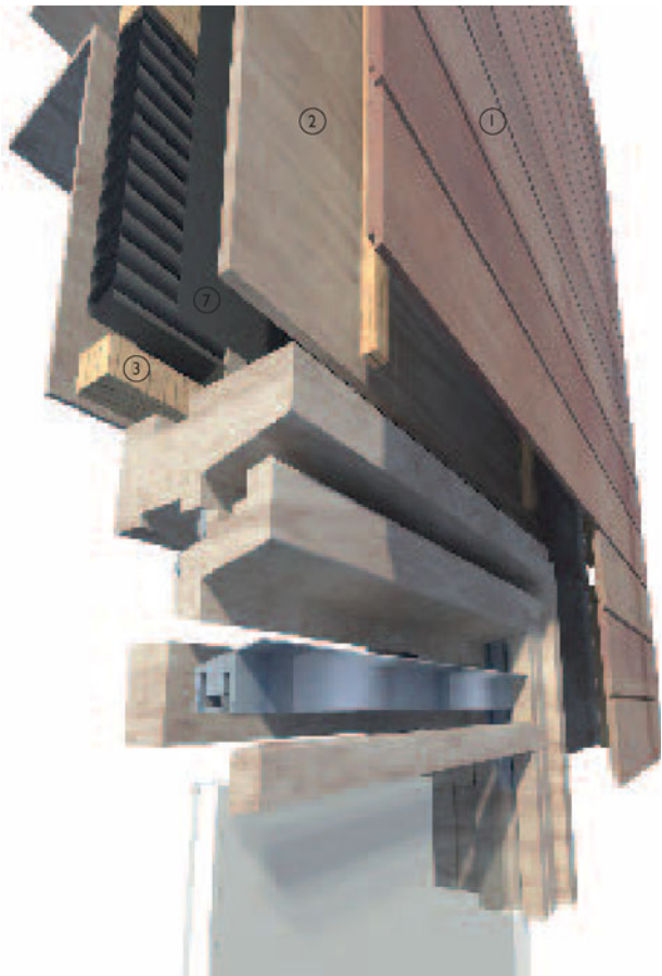
3-D exploded detail view of top of window opening in timber cladding system
