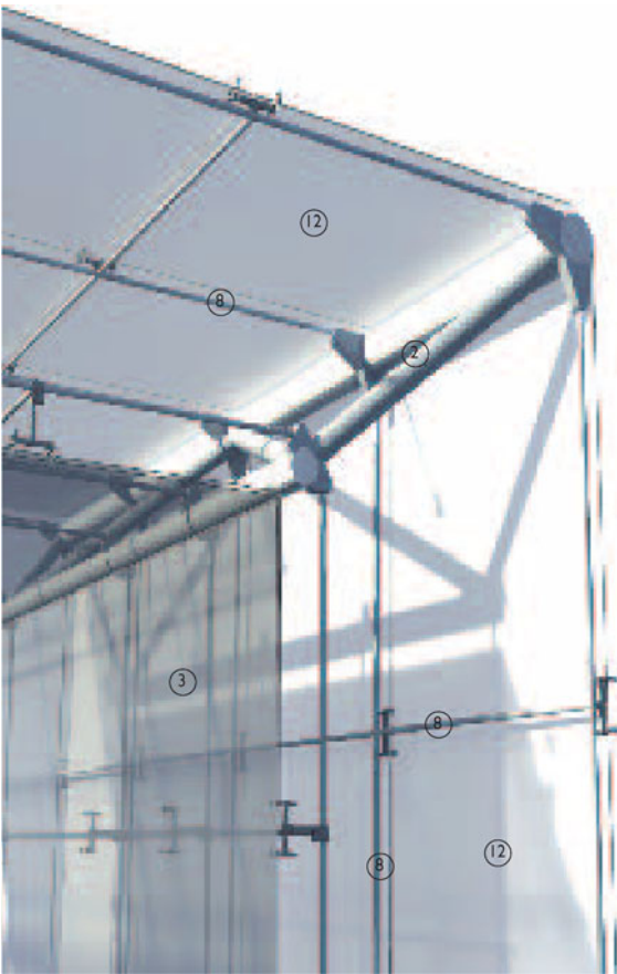
3-D view showing fixing method of twin wall roof with double glazed units, steel truss support system and glazed solar shading
