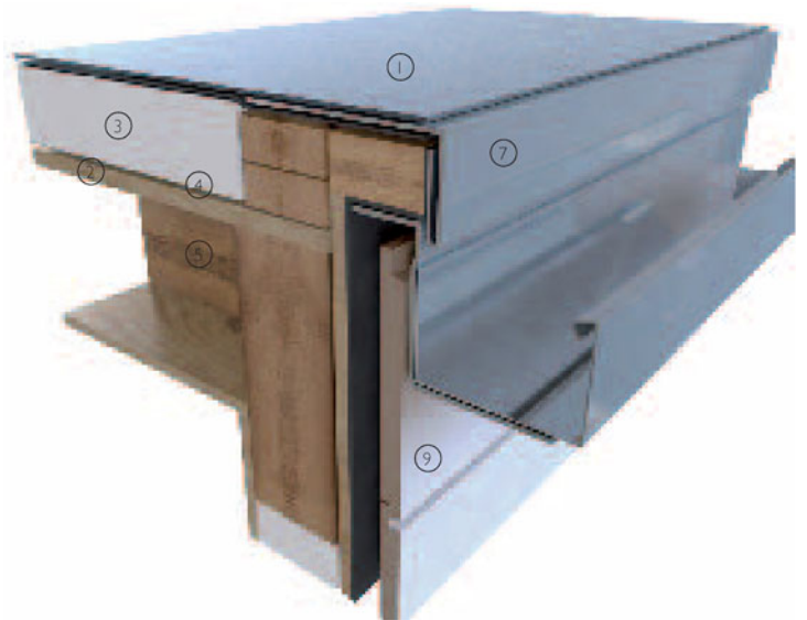
3-D view of flat roof with a bitumen-based sheet membrane, eaves detail
