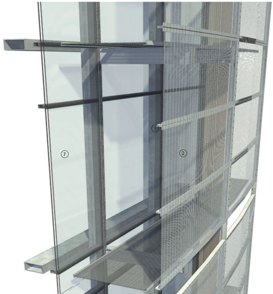
3-D view of metal mesh fixed in front of glazed facade to provide solar shading. A maintenance walkway occupies the space between the two systems
