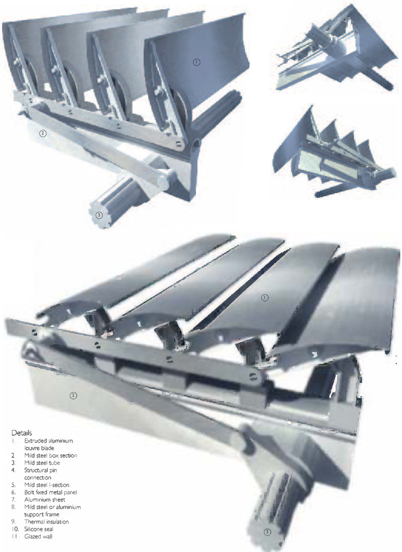
3-D views of electrically operated louvre panel in open and closed positions
