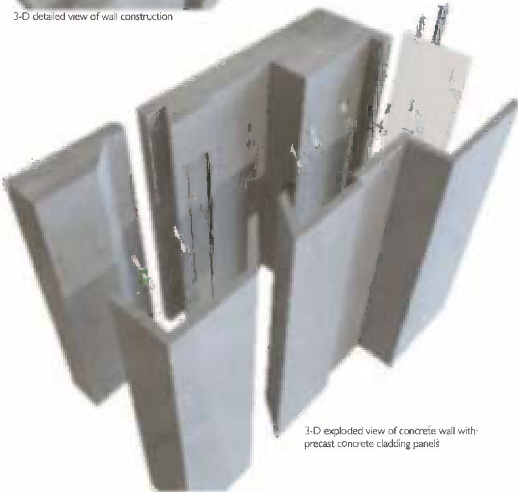
3-D detailed view of wall construction
