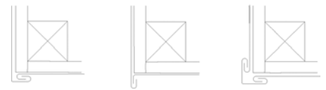
Horizontal section 1:10. Simple seam details at corners
