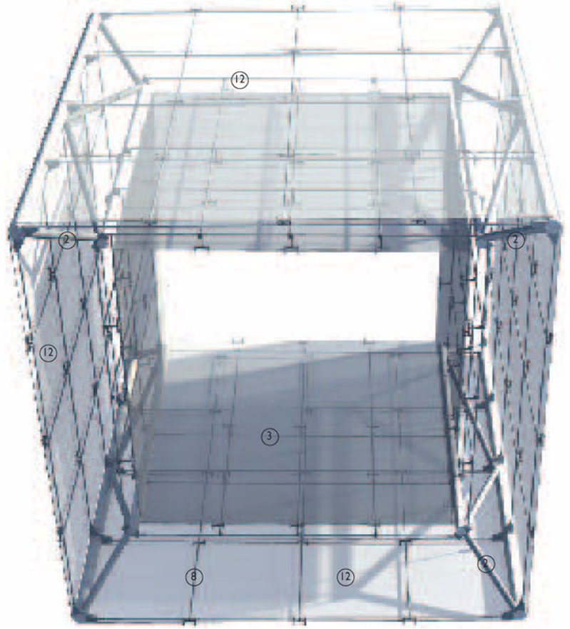
3-D view showing overview of twin wall roof with double glazed units, steel truss support system and glazed solar shading
