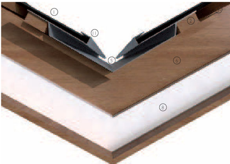
3-D view of valley detail in timber pitched roof construction with roofing slates
