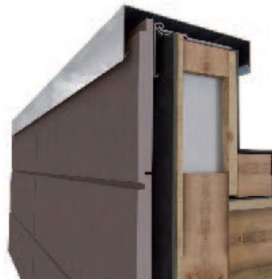
3-D view of flat roof with a bitumen-based sheet membrane, parapet detail
