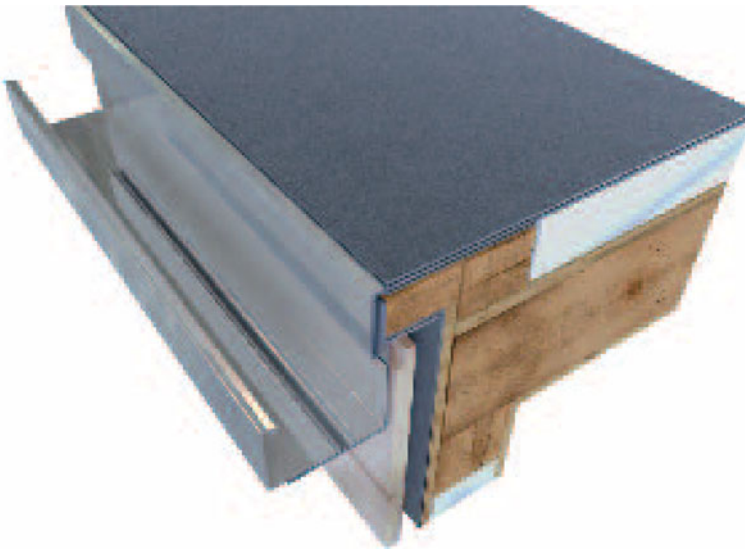
3-D view of flat roof with a bitumen-based sheet membrane, eaves detail
