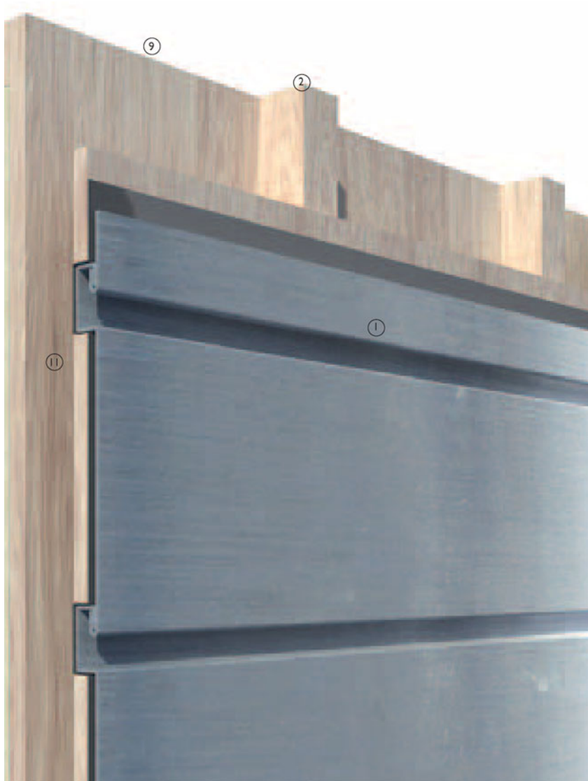
3-D view of folded metal sheet with recessed seams. Type I
