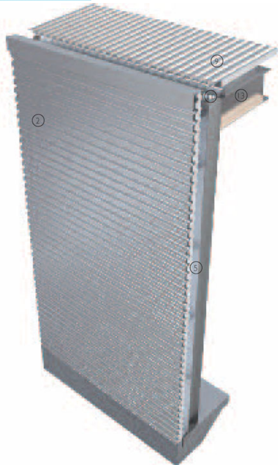
3-D view of horizontally set profiled metal sheet
