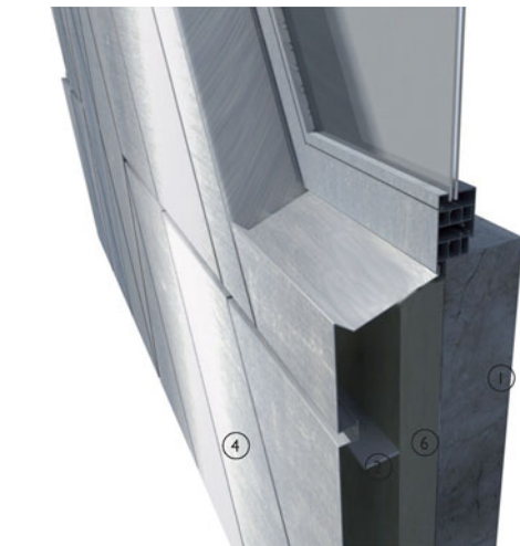
3-D view of semi interlocking metal rainscreen with angled joints and aluminium window recessed into the facade. Type 3
