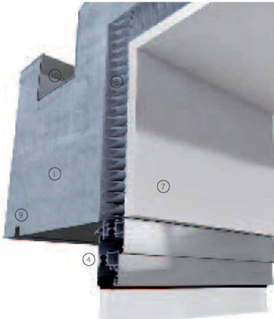
3-D view of parapet junction of an in-situ cast concrete wall cast as a monolithic construction with internal thermal insulation
