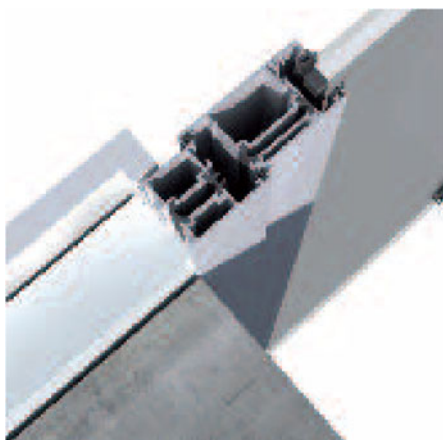
3-D detail view of window jamb in an in-situ cast concrete wall cast as a monolithic construction with internal thermal insulation
