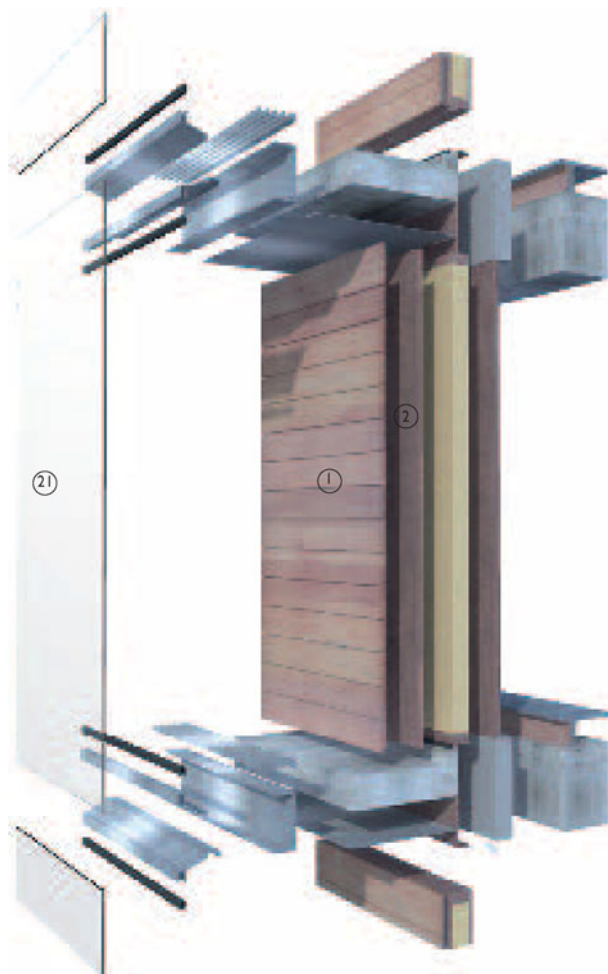
3-D exploded view of cladding panel in twin wall configuration for taller buildings
