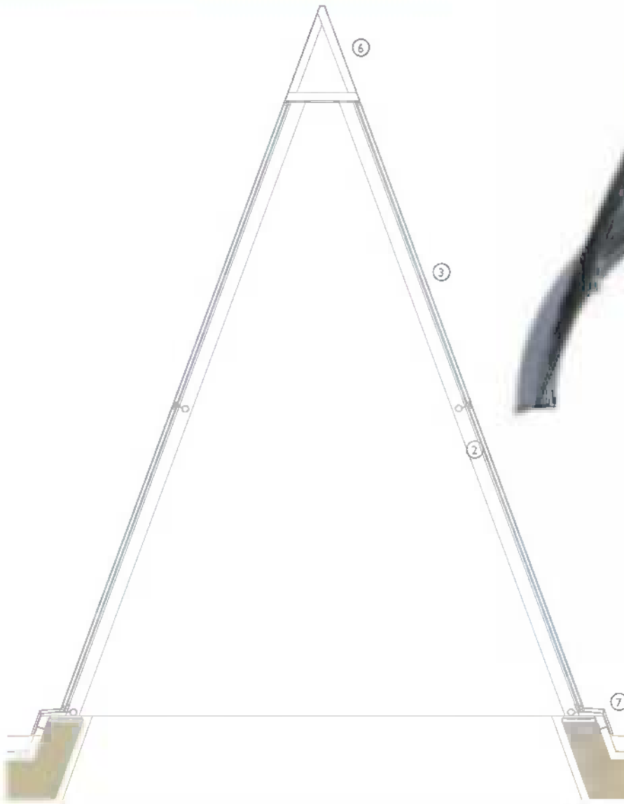
Vertical section 1:25. Generic conical rooflight, typical assembly
