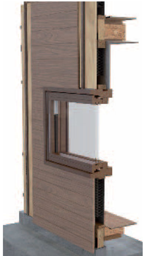
3-D view of timber wall construction
