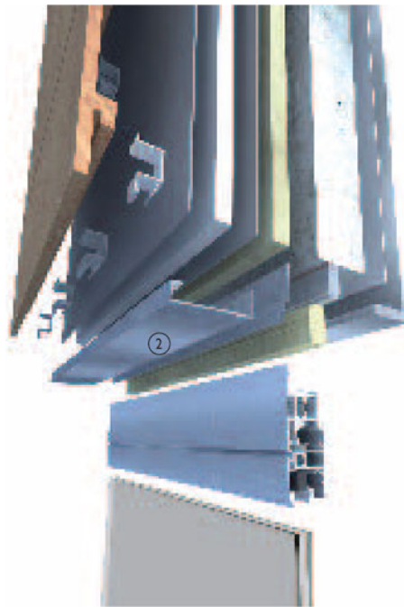
3-D exploded view of top of window opening in terracotta rainscreen wall assembly
