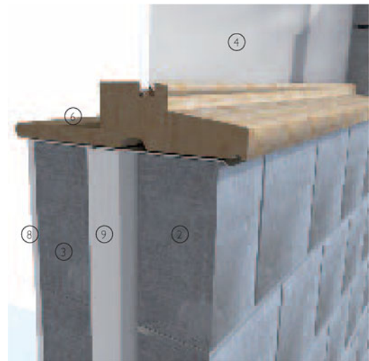
3-D view of window cill detail
