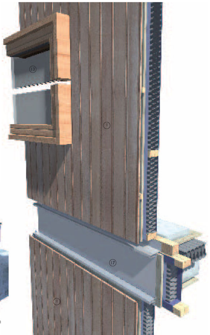
3-D view of cladding panel assembly with built-in opening window
