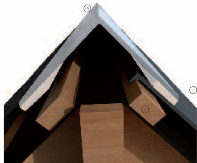
3-D view of ridge detail of timber pitched roof construction with roofing slates
