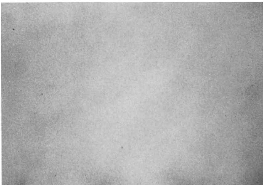
Figure 4.5 Optical photomicrograph of liquid ink exhibiting no flocculation of pigment particles.
