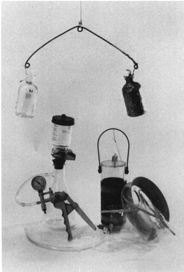
Fig. 1.2.2 Some field equipment used in the assessment of eutrophication: a cylindrical water sampler equipped with trapdoors and cord; filter assembly and pump; a pair of light and dark bottles, several of which may be connected in series; plastic sample bags. (Photo: John Watson)
