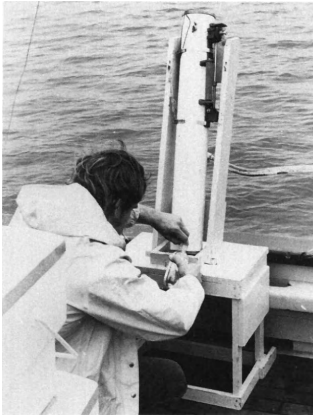
Fig. 1.1.3 Water samples are run from a sampling device used to collect water at depth. Analyses for dissolved oxygen are subsequently carried out in the laboratory.
