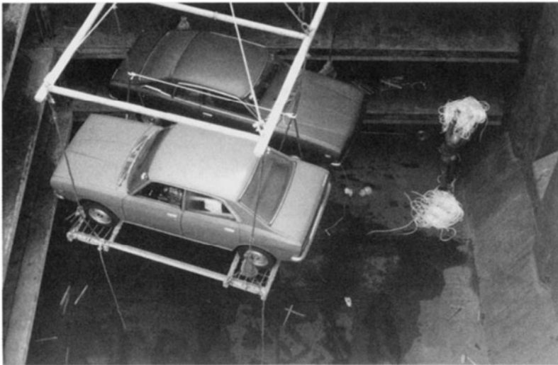
A dry bulk carrier converted to carry cars, 1976 (photograph WWL Archive)
