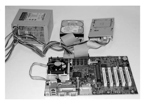
You can find processors, RAM, the motherboard chipset, and motherboard BIOS on the motherboard. The chipset represents the nerve clusters that connect your various components including the keyboard, disk drives, and RAM. Depending on the design of the motherboard, one chipset may run faster than another chipset or have more redundant features. Of course, these types of systems usually cost more.
