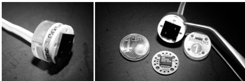
Fig. 9.5 Microstructured pressure/temperature sensor made of silicon for flow-through applications [30].
