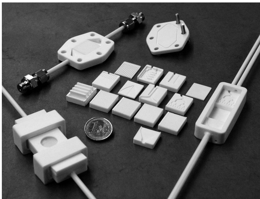
Fig. 12.7 Different designs of ceramic microreactors with a variety of exchangeable inserts ([33] – reproduced by permission of The Royal Society of Chemistry).
