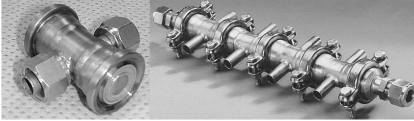
Fig. 6.14 Microstructured reactor module. Length: 60 mm (left) and the assembled microreactor. Length: 240 mm, total reactor volume: 3 cm 3 (right) [22].
