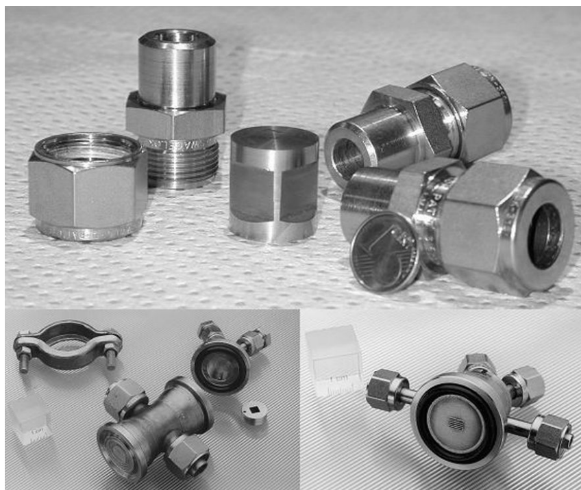
Fig. 10.40 Top: Size comparison between the central core of a crossflow microchannel heat exchanger ( 1 \text{ cm}^3 active volume) to three standard fittings used for adaptation (about 2.9 \text{ cm}^3 each). Bottom left: micro-mixer and microchannel reactor/heat
