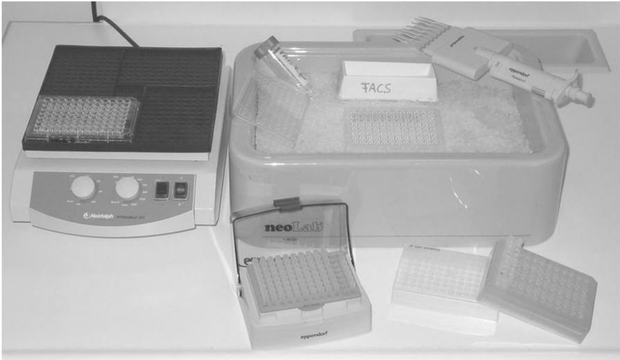
**Fig. 1.** Necessary equipment to perform a staining procedure: 96-well round bottom microtiter plates, microtiter plate shaker, ice bath, 8- or 12-channel pipette, buffer reservoir for multichannel pipette, minitubes, and minitube rack (96-well format)
