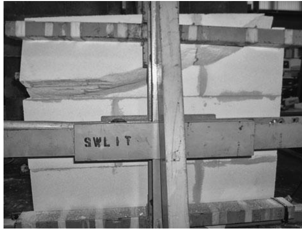
Figure 13.5 Failure of an aircrete wall using conventional mortar under four-point loading
