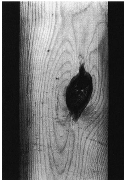
Figure 16.6 A 'dead' knot. The knot is separated from the wood of the trunk by a layer of bark (BRE © Crown copyright)
