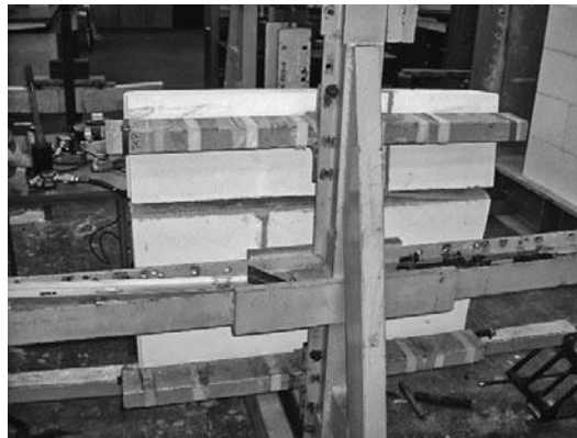
Figure 13.6 Failure of an aircrete wall using thin layer mortar under four-point loading
