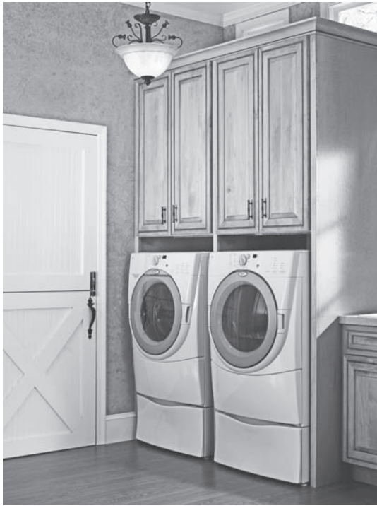
Figure 7-2 Kitchen cabinet manufacturers make laundry room cabinets that are similar to kitchen cabinets in size and construction. In addition, cabinets in special sizes and with special laundry-related fittings such as hampers and foldout ironing boards are available. The wall cabinets shown are deeper and taller than standard kitchen wall cabinets, to accommodate a front-loading washer and dryer on a pedestal.
