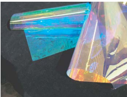
▲ Figure 1-5 Radiant color film. The color of the transmitted or reflected light depends upon the vantage point. Observers at different places would see different colors (see Chapter 6)
