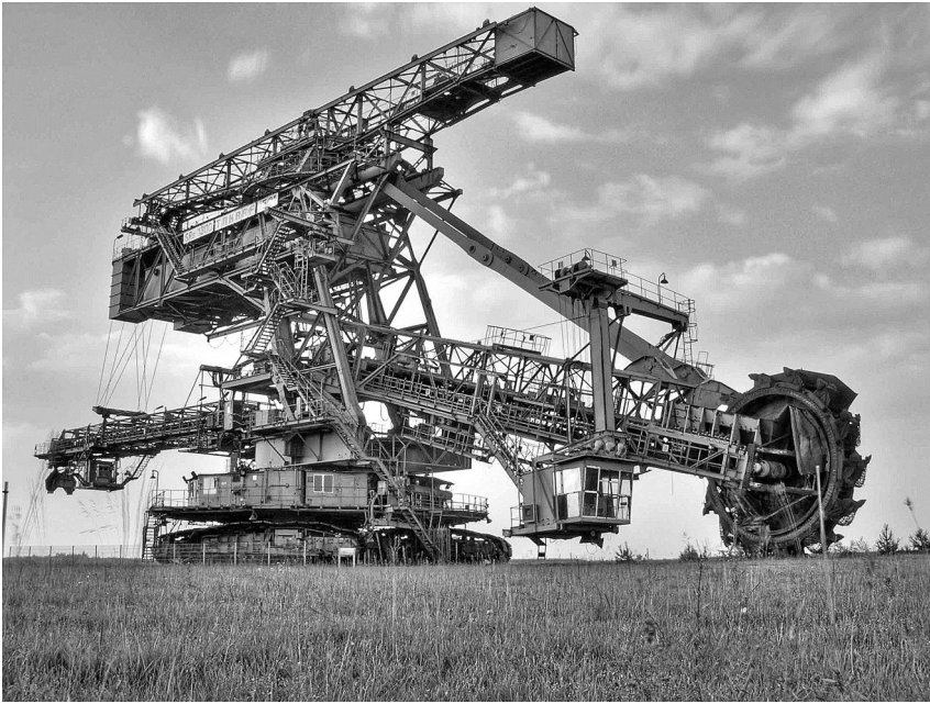
FIGURE 3.3 Bucket wheel excavator in Ferropolis. Courtesy of Rmollik under Creative Commons License.
