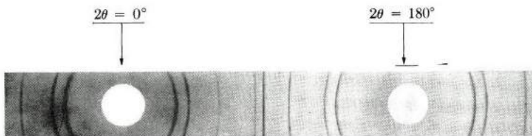
Fig. 2.15 The x-ray powder diffraction pattern for Cu. 2\theta is the scattering angle. [After Cullity (1956)]
