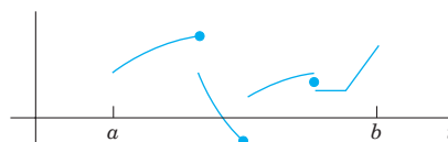
Fig. 115. Example of a piecewise continuous function f(t) . (The dots mark the function values at the jumps.)
