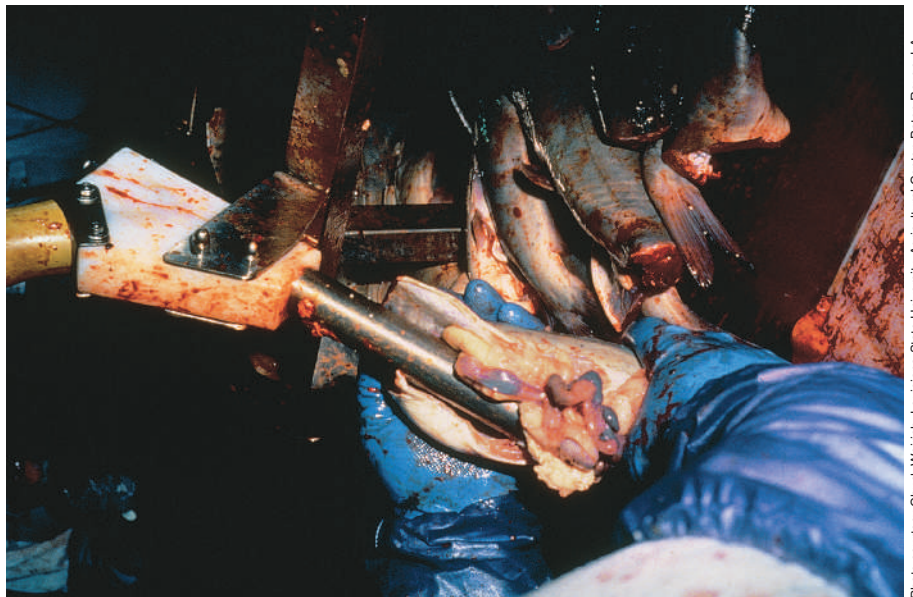
Figure 3-13 Removing viscera from the body cavity of the fish with a vacuum eviscerator.
