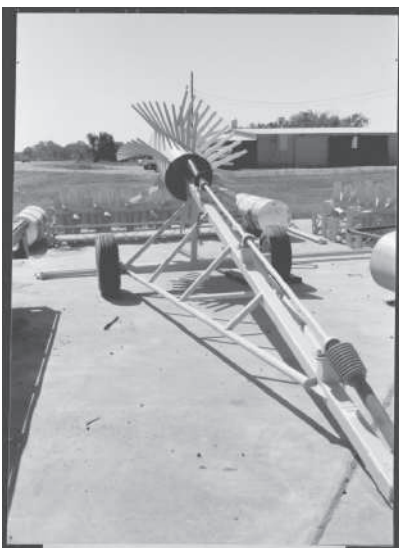
FIGURE 13-22 Side wheel style paddlewheel aerator. This aerator requires the PTO of a 45-hp tractor.
