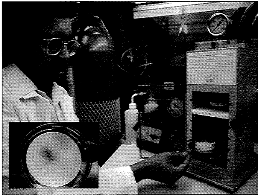
Figure 4.2 A researcher uses a gene gun to introduce new genes into an organism. DNA is coated onto microscopic gold or tungsten pellets that are propelled by the particle gun into plant or animal tissues that are in a petri dish (inset).
