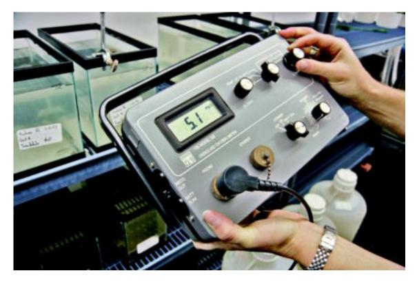
Chemist using an oxygen meter to perform a bioassay test. Bioassays are sometimes used to measure how well a drug is working in a biological system. © Bob Rowan: Progressive Image/ Corbis.
