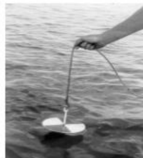
Fig 6.1. (a) A secchi disc with its cable (b) A secchi disc lowered into water body
