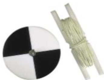
Fig 6.1. (a) A secchi disc with its cable (b) A secchi disc lowered into water body
