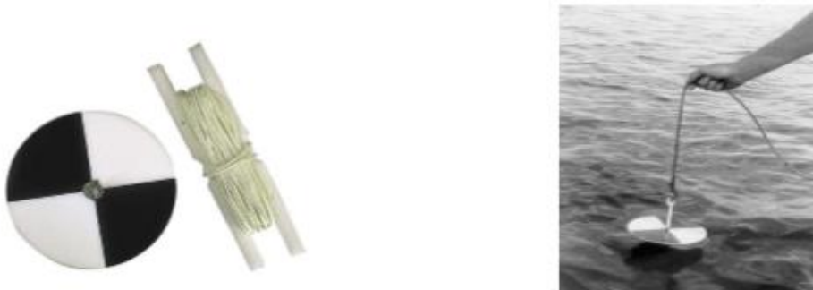
Fig 6.1. (a) A secchi disk with its cable (b) A secchi disk lowered into water body
