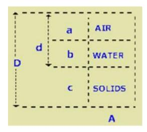
A cube of soil measures 10 cm x 10 cm x 10 cm (D = 10 cm, A = 100 sq cm) and has a total wet mass of 1990 g of which 280 g is water. Assume the density of water is 1 g per cc and particle density is 2.65 g per cc. Find the depth of water, water-holding capacity and aeration porosity of the soil.
