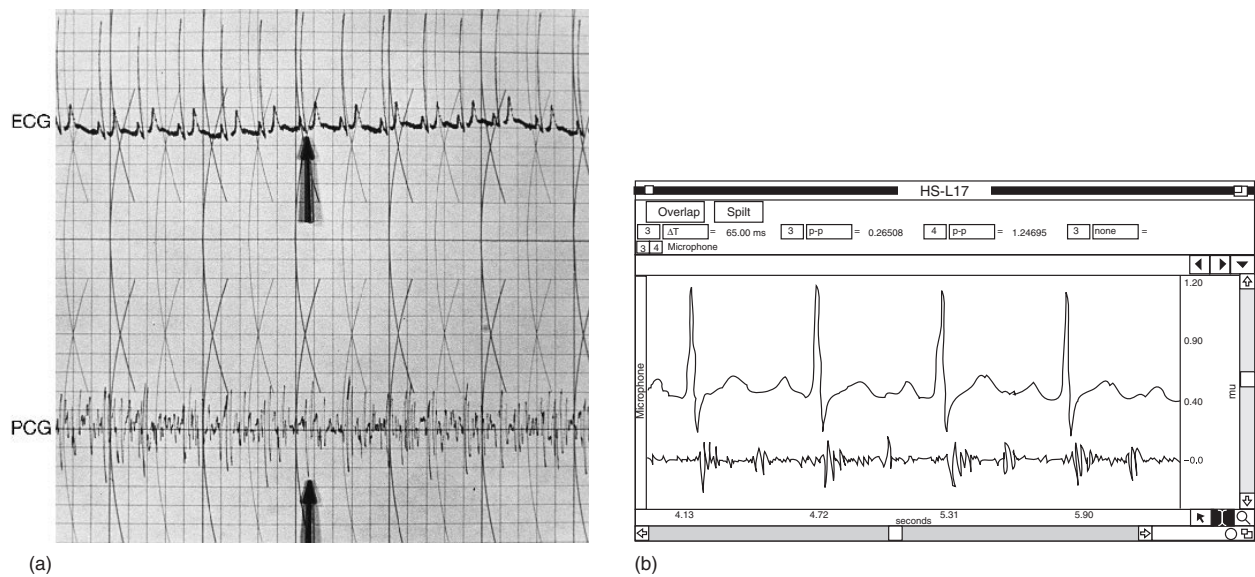
Figure 7.20 Simultaneous recording of an electrocardiogram (ECG) and a phonocardiogram (PCG). (a) Photograph of recordings taken with a Narco physiograph. (b) Idealized computer image of recordings taken with the Biopac system ECG electrodes and amplified stethoscope.
