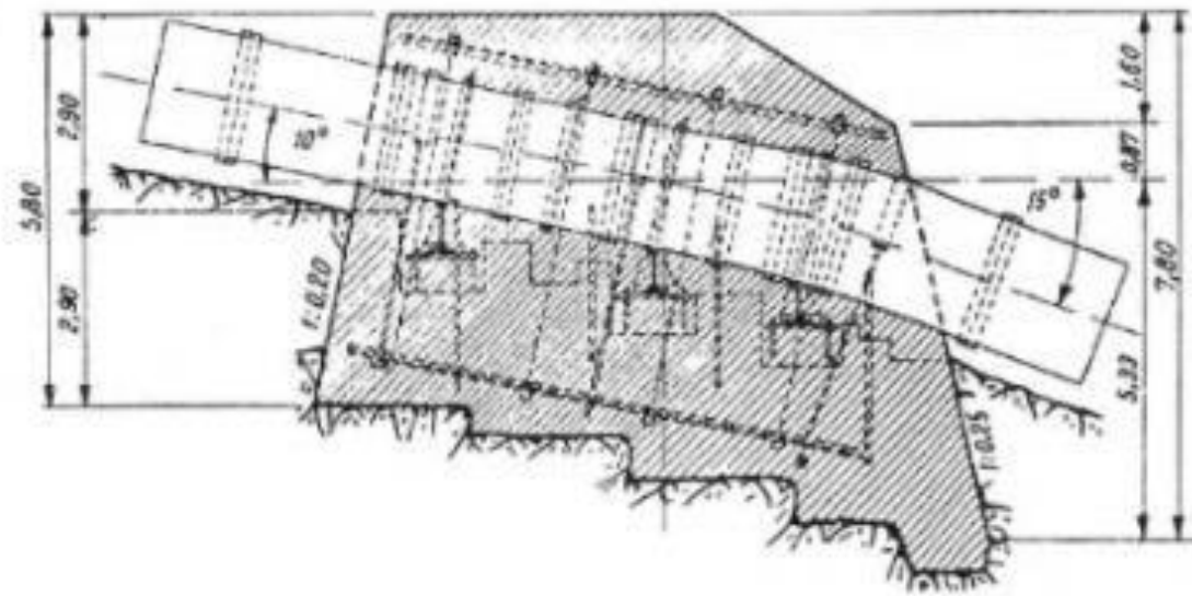
Fig. 4/93. Anchor detail showing hold-down straps for penstock, Arnstein power plant. (After A. Schoklitsch)
