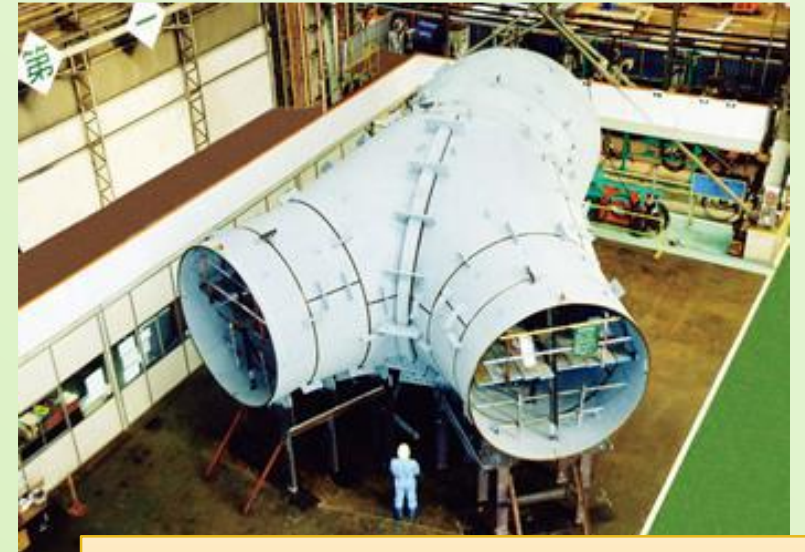
A penstock bifurcation under production at a fabrication plant Courtesy of Mitsubishi Heavy Industries, Ltd., Japan
