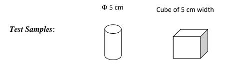
*Test procedure*: Test shall be carried on *saturated* as well as on *dry samples* Saturated: immerse samples in water at 20-30°C for 72 hrs and then test in saturated condition. Dry: oven dried at 105+5°C for 24 hrs. Then cooled in a desiccator to room temperature.
