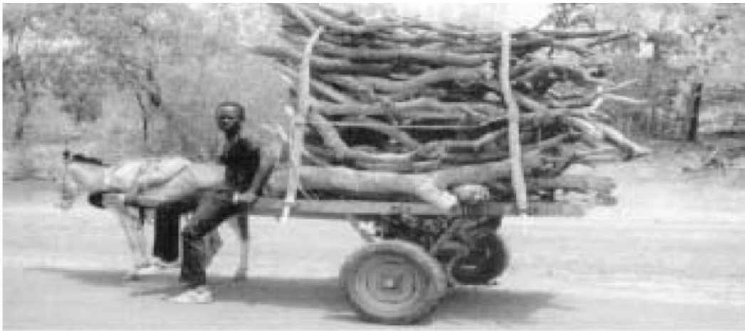
Figure 30: Two-wheel donkey cart in Mali. Provided the load is well balanced, donkeys can pull impressive loads along flat roads.
