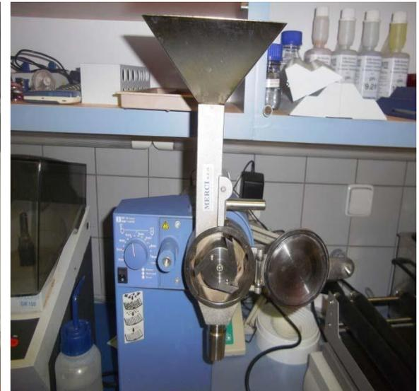
Weighing plant specimen and grinding it using Grindo mix
