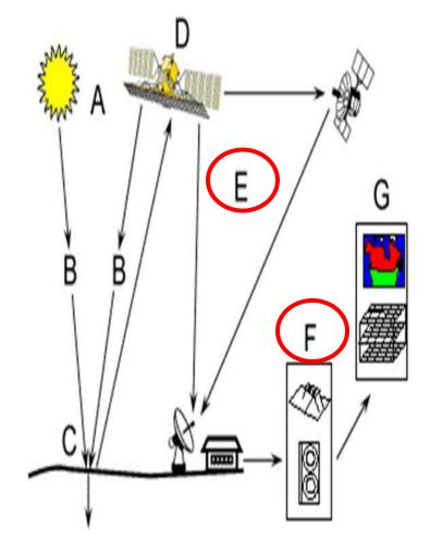
Application (G) - the final element of the remote sensing process is achieved when we apply the information we have been able to extract from the imagery about the target in order to better understand it, reveal some new information, or assist in solving a particular problem.
