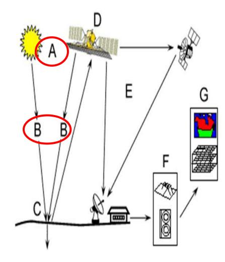
Interaction with the Target (C) once the energy makes its way to the target through the atmosphere, it interacts with the target depending on the properties of both the target and the radiation.
