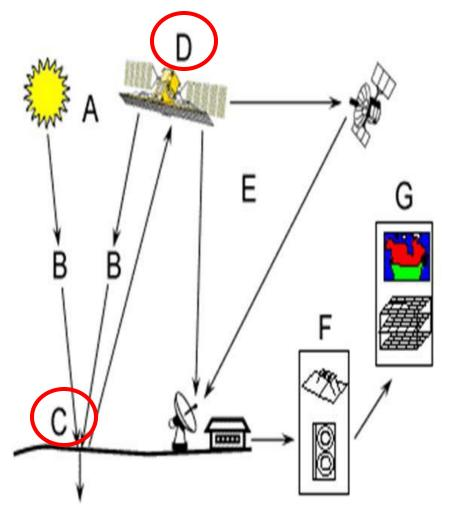
**Reception, and Processing (E)** - the energy recorded by the sensor has to be transmitted, often in electronic form, to a receiving and processing station where the data are processed into an image (hardcopy and/or digital).
