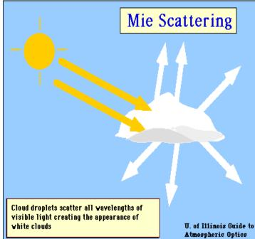
Non-selective scattering occurs when particle sizes are much larger than the radiation wavelength. Typical particles responsible for this effect are water droplets and larger dust particles.
