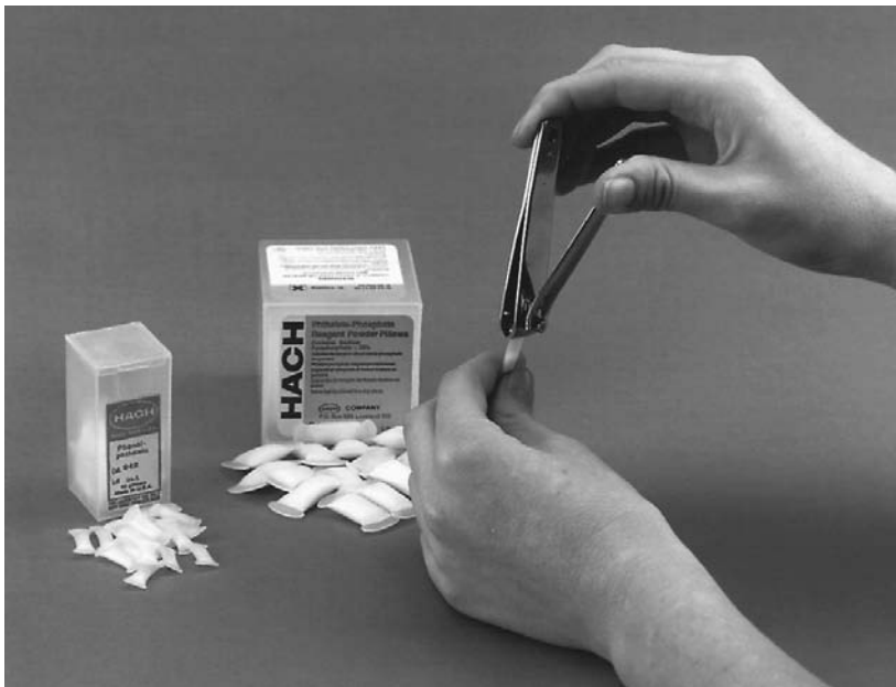
Figure 7 Opening Powder Pillows
