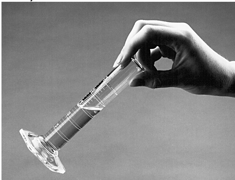
Figure 5 Swirling a Graduated Cylinder
