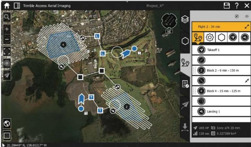
**FIGURE 7.28** UX5 HP flight plan. (Courtesy of Trimble.)
