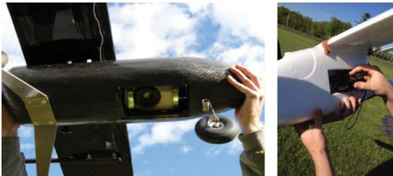
**FIGURE 7.4** Sensors installed at Michigan Tech in UAV (Canon Reibel EOS) and E38 small UAV (Canon SX 260 HS).
