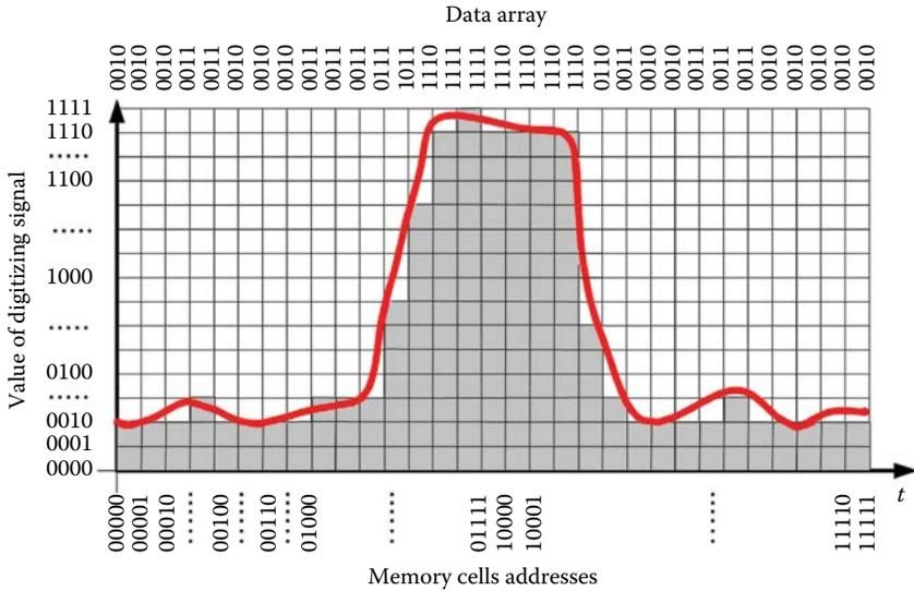
**FIGURE 4.16** Digitalization of an analog signal.
