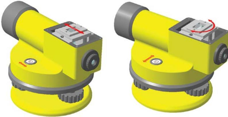
**FIGURE 2.20** Adjusting of compensator position.
