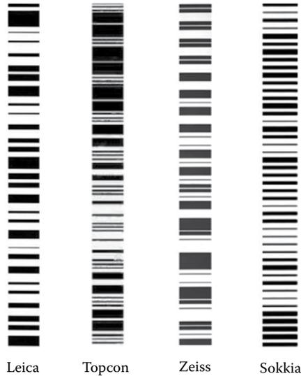
**FIGURE 2.24** Rods for digital levels.
