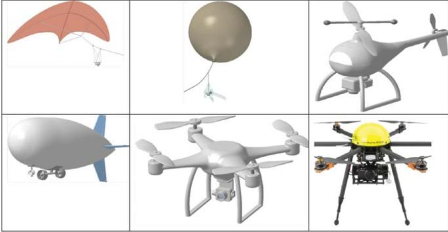
**FIGURE 7.1** Different surveying UAV platforms.
