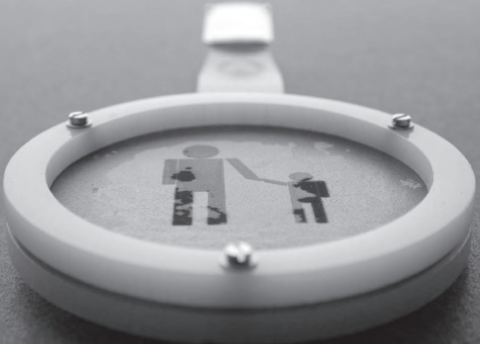
Effect of laser through graphite onto titanium.
