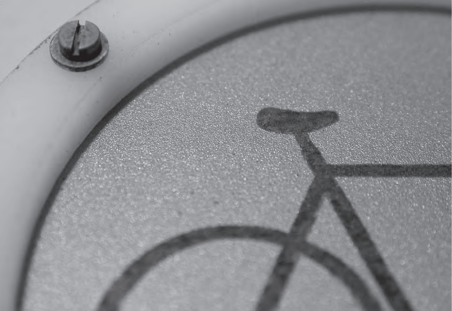
Laser marked titanium.
