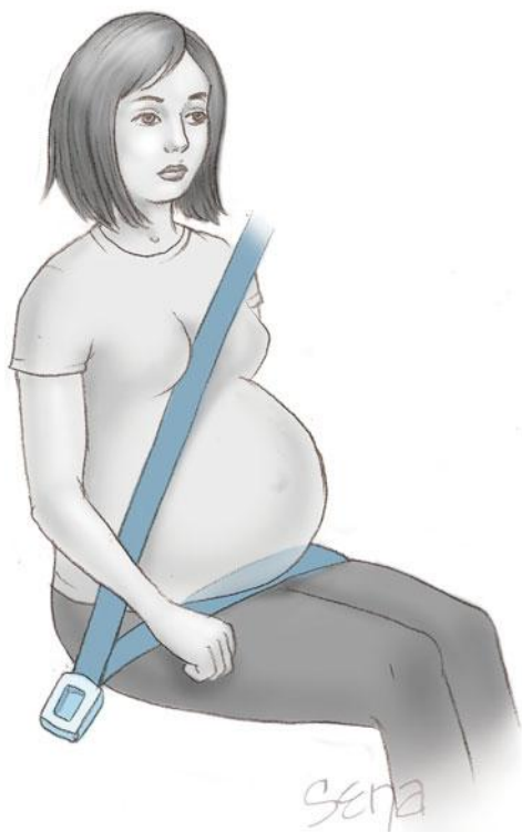
FIGURE 47-8 Illustration showing correct use of three-point automobile restraint. The upper belt is above the uterus, and the lower belt fits snugly across the upper thighs and well below the uterus.
