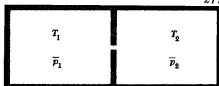
Fig. 7-12-4 A container divided into two parts by a partition containing a small hole. The gas in the two parts is at different temperatures and pressures.
