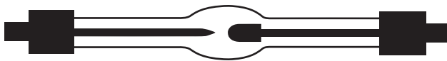
Figure 5.55 Compact xenon arc lamp used in fluorometers. The quartz envelope is filled with xenon gas. The lamp is ignited by a 10–20 kV pulse across the electrodes. (From Froelich, P.M. and Guilbault, G.G., In Practical Fluorescence , 2nd edn., Guilbault, G.G., ed., Marcel Dekker, Inc., New York, 1990. With permission.)
