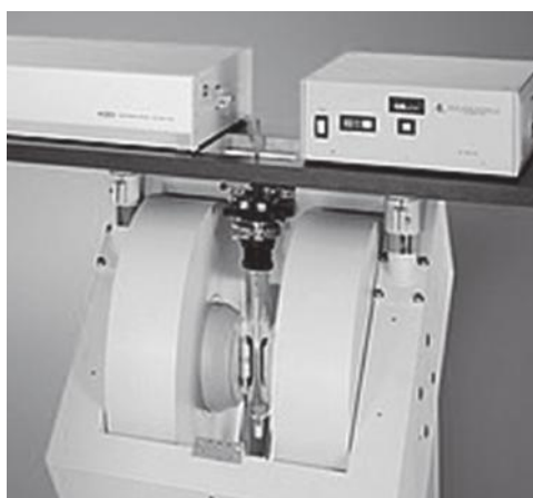
Figure 3.80 (continued) (c) Simulated absorbance spectrum and its first derivative. ESR spectra are plotted as first derivative spectra. (d) Bruker ELEXSYS-II EPR. (Courtesy of Bruker Corporation, www.bruker-biospin.com .)
