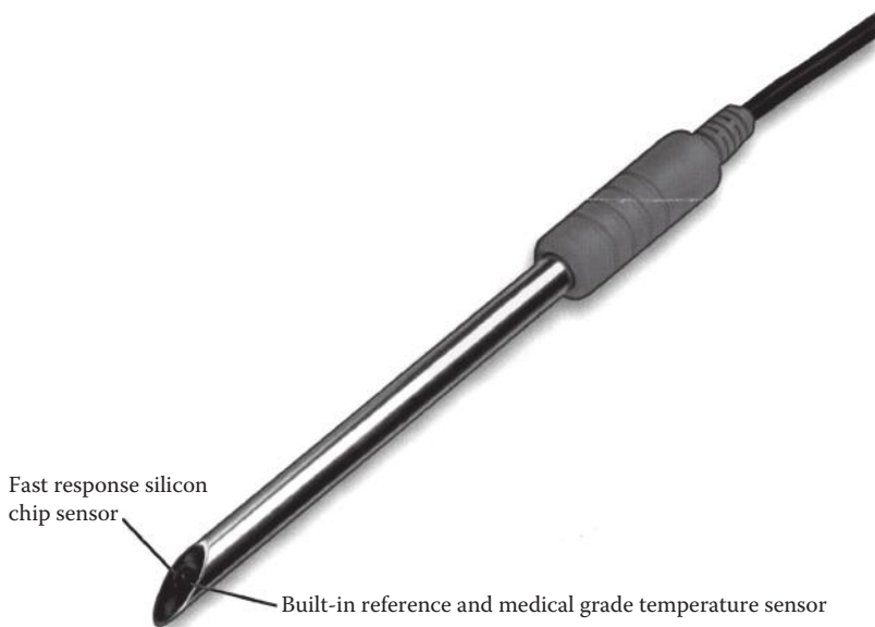
Figure 15.12 A commercial ISFET pH probe, with a silicon chip pH sensor, a built-in REF, and a built-in temperature sensor. This pH probe is housed in a stainless steel body with a slanted tip for easy insertion into meat or other soft solid samples. (Courtesy of IQ Scientific Instruments, Inc., Carlsbad, CA.)
