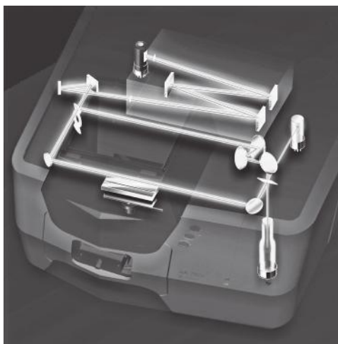
Figure 6.14 (a) Schematic double-beam AAS configuration. [© 1993–2014 PerkinElmer, Inc. All rights reserved. Printed with permission. (www.perkinelmer.com).] (b) The optical path of the Shimadzu Scientific Instruments AA-7000 superimposed over the actual instrument body. On the right, from front to back is the HCL, the beam splitter (slanted rectangle) and the deuterium lamp. In the center, from front to back, we have the burner head with the sample beam passing over it, the reference beam, and the monochromator at the center top. On the left is the mirrored chopper and in the back, the detector. (Courtesy of Shimadzu Scientific Instruments, Inc. www.shimadzu.com.)
