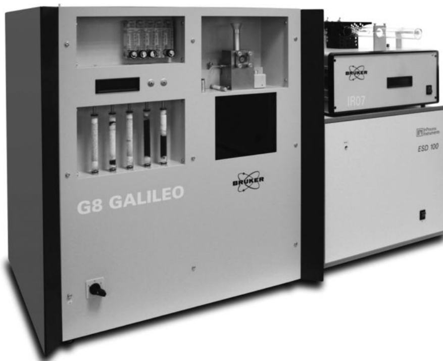
Figure 10.40 The Bruker G8 Galileo O/N/H analyzer, equipped with a quadrupole mass spectrometer detector (lower right) and an external IR furnace (upper right) for diffusible hydrogen. (© 2013 Bruker Corporation, www.bruker-axs.com . Used with permission.)
