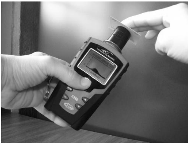
Figure 5.37 The i-LAB ® Visible Hand Held Analyzing Spectrometer measuring a solid sample. (Courtesy of Microspectral Analysis, LLC, Wilton, ME, www.microspectralanalysis.com .)
