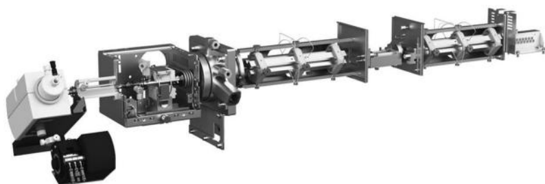
Figure 10.43 The Agilent Technologies 8800 ICP-QQQ. From the left, sample introduction, the ICP torch box (note the cooling coils for the torch), Q1, the ORS 3 octopole collision/reaction cell, Q2, and finally, the electron multiplier detector. (© 2014 Agilent Technologies, www.agilent.com/chem. All rights reserved. Used with permission.)
