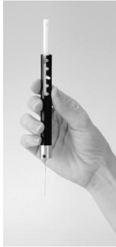
Figure 1.11 An SPME probe the size of a ball-point pen. (Reprinted with permission of Supelco, Bellefonte, PA. www.sigma-aldrich.com .)
