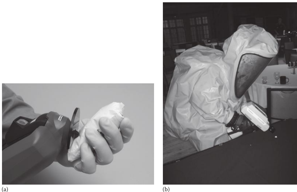
Figure 4.69 (a) Handheld TruScan® Raman instrument collecting a spectrum from a powder sample directly through the plastic bag. (© Thermo Fisher Scientific ( www.thermofisher.com ). Used with permission.) (b) Hazardous material identification by a first responder using the handheld FirstGuard™ 1064 nm advanced Raman system. (Used with permission of Rigaku Raman Technologies, Inc., www.rigakuraman.com .)
