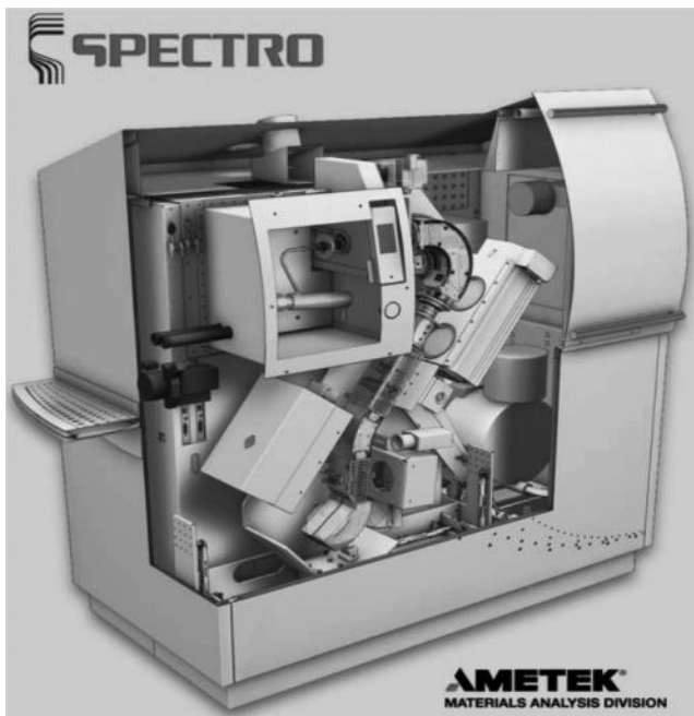
Figure 9.24 Cutaway view of the SPECTRO MS, showing the ICP torch box upper left and the ion optic to the right of the torch box, leading to the mass spectrometer on the left under the torch box. (Courtesy of SPECTRO Analytical Instruments, Inc., AMETEK® Materials Analysis Division. www.spectro.com, www.ametek.com. Used with permission.)
