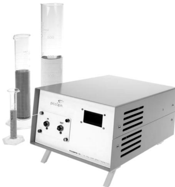
Figure 3.74 The miniature picoSpin-45 proton NMR. (Used with permission of picoSpin, LLC, www.picospin.com .)
