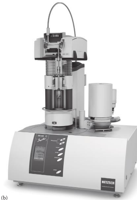
Figure 16.29 (Continued) (b) The Perseus TGA-DSC-FTIR system with a vertical arrangement of the FTIR and thermal analysis system, with no external transfer line. (Courtesy of NETZSCH Instruments, Inc., Burlington, MA, www.netzsch-hermal-analysis.com .)
