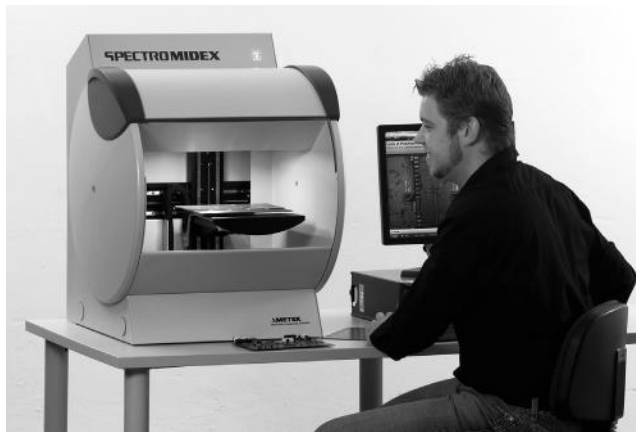
Figure 8.46 A micro-XRF system with a large sample chamber, the SPECTRO MIDEX. This is used for analysis of large objects, such as the complete circuit board shown to the left of the analyst. (© AMETEK, Inc. www.ametek.com. Used with permission.)
