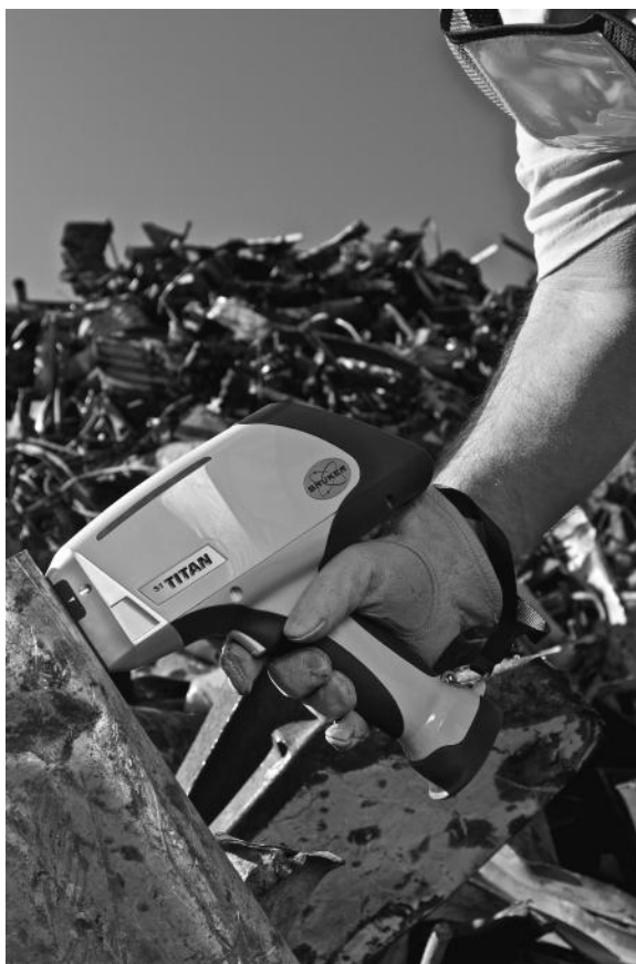
Figure 8.54 Scrap metal sorting using the TITAN, an HH XRF analyzer, to identify elemental composition. (Courtesy of Bruker Elemental, © 2013 Bruker, Inc. www.bruker.com . Used with permission.)
