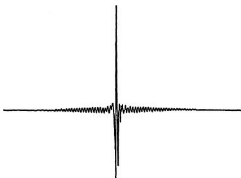
Figure 4.12 An idealized interferogram. (From Coates, J., Vibrational spectroscopy , in Ewing, G.W., ed., Analytical Instrumentation Handbook , 2nd edn., Marcel Dekker, Inc., New York, 1997. With permission.)
