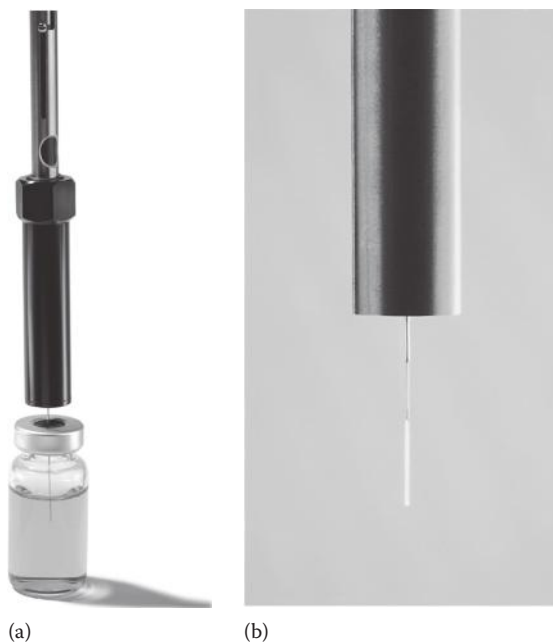
Figure 1.9 (a) A commercial SPME unit with (b) the coated fiber and inserted into a sample vial. (Reprinted with permission of Supelco, Bellefonte, PA, www.sigma-aldrich.com.)
