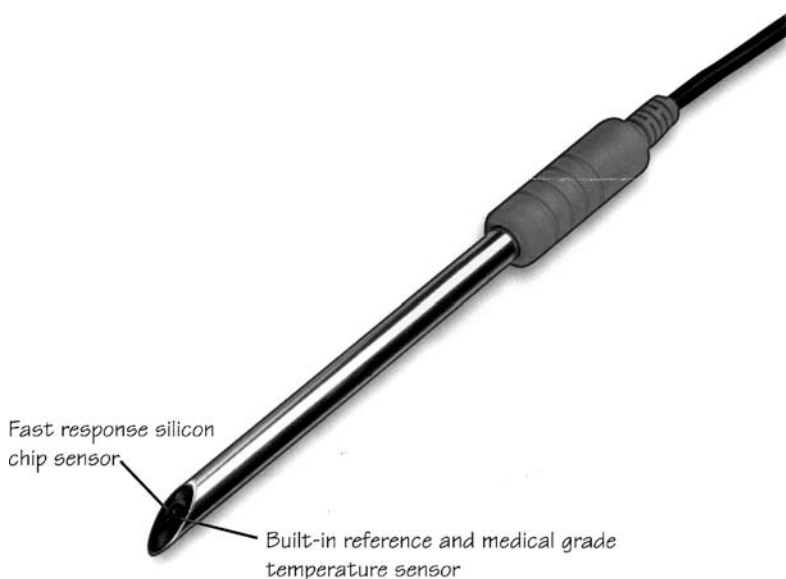
Figure 15.12 A commercial ISFET pH probe, with a silicon chip pH sensor, a built in reference electrode, and a built-in temperature sensor. This pH probe is housed in a stainless steel body with a slanted tip for easy insertion into meat or other soft solid samples. (Courtesy of IQ Scientific Instruments, Inc. San Diego, CA.)
