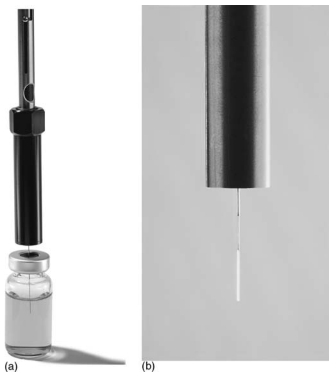
Figure 1.9 (a) A commercial SPME unit with the coated fiber (b) inserted into a sample vial. Reprinted with permission of Supelco, Bellefonte, PA 16823, USA ( www.sigma-aldrich.com ).
