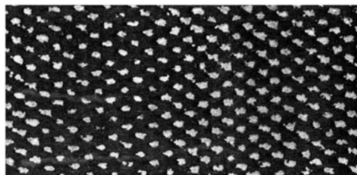
Figure 8.35 An electron micrograph of the (110) plane in crystalline silicon.
