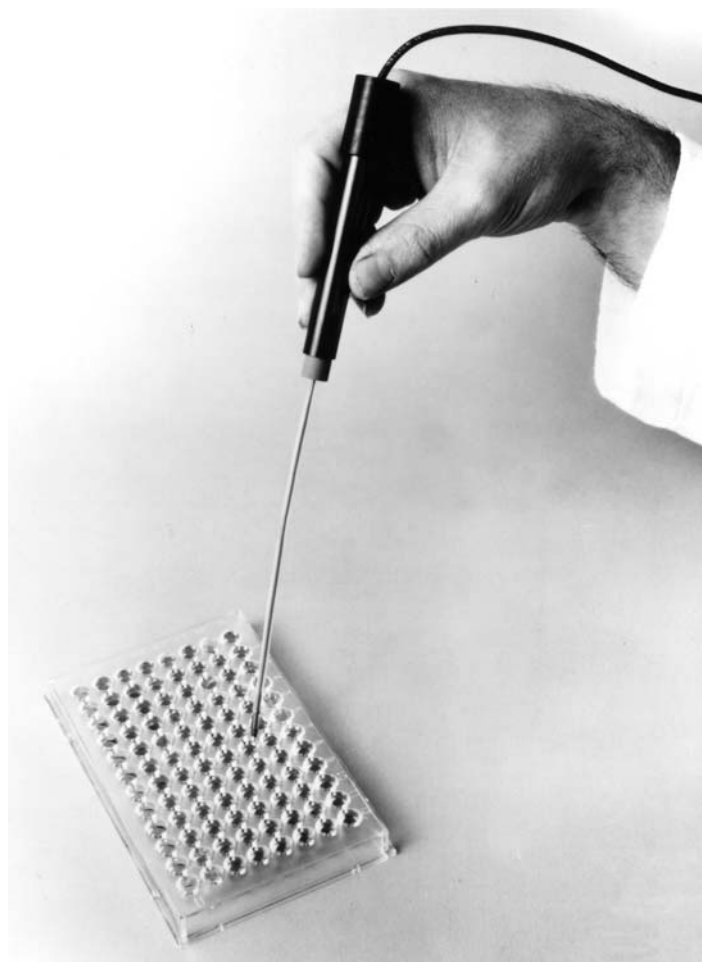
Figure 15.8 A commercial microelectrode for pH measurements in volumes as small as 10 \mu\text{L} . The electrode has a solid-state pH sensor and a flexible polypropylene stem, making it extremely rugged and suitable for use in the field. This electrode can be used to determine pH in single droplets of water on leaves of plants or blades of grass to study acid rain deposition. [Courtesy of Lazar Research Laboratories, Inc., Los Angeles, CA ( www.lazarlab.com ).]
