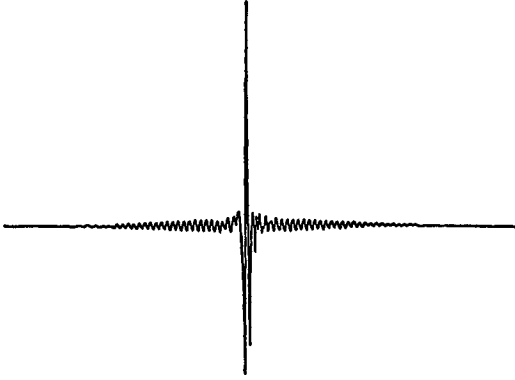
Figure 4.12 An idealized interferogram. (From Coates, used with permission.)
