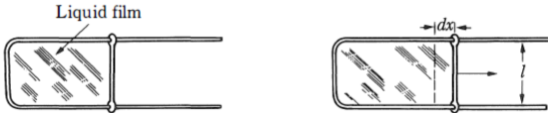
Figure: A soap film stretched across a wire frame with one movable side.
