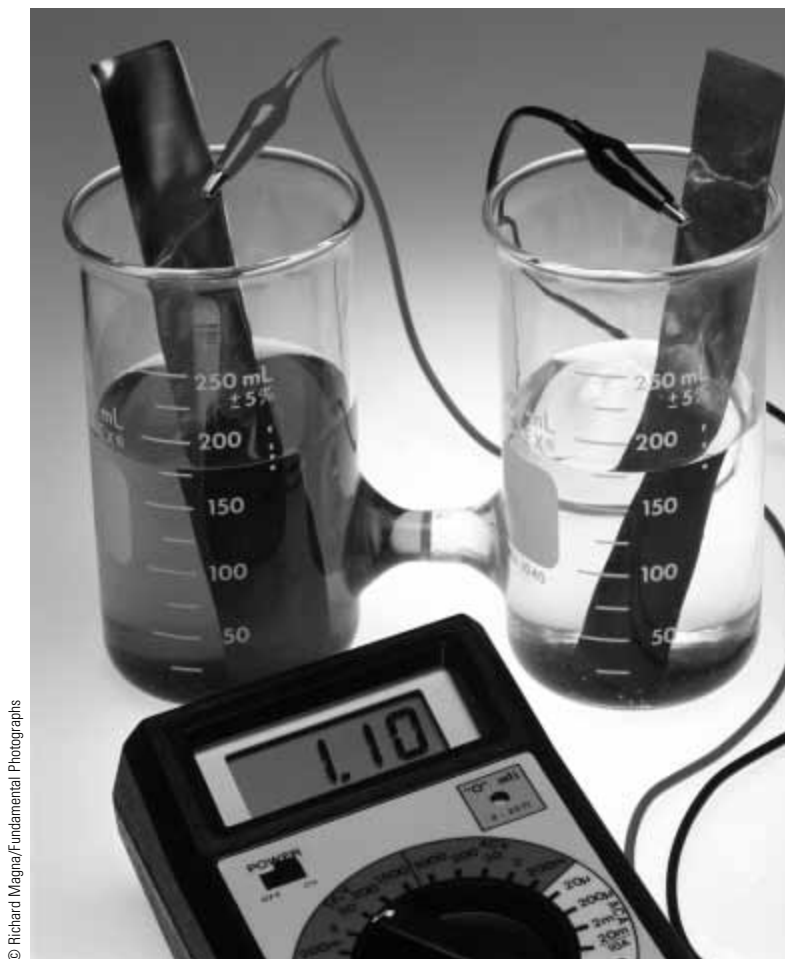
Figure 8.3 The same redox reaction as in Figure 8.2 is shown, but now each half-reaction is physically separate from the other. As this redox reaction occurs, we can extract useful work from the transfer of electrons, as shown.
