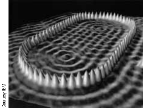
Figure 10.11 An STM image of a ring of Fe atoms on a copper surface.
