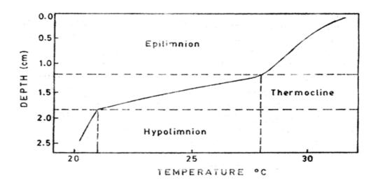
Fig 1.2. An Illustration of Thermal Stratification
