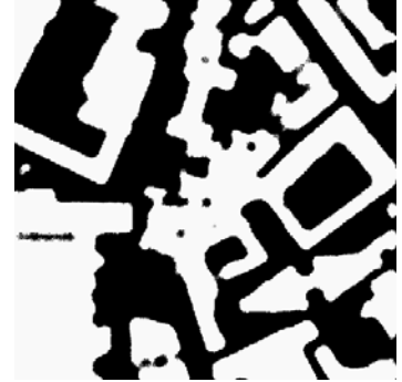
6.13 Wind shadow map where black areas indicate areas predominantly in wind shadow
