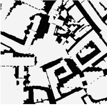
6.11 Shadow map of Cambridge, where black zones are those that receive less than 6 hours of sunlight on 22 June when the theoretical maximum is 15 hours
