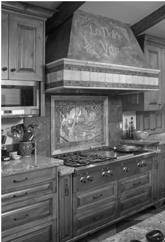
Figure 5-23 The advantage of the range top over the full range is the option of placing the range top at the proper height for the cook. (Photo courtesy of Mary Fisher Designs.com and Northlight Architectural Photography.com)
