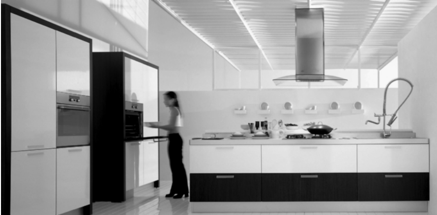
Figure 3-6 The installation height of the oven(s) enables the cook to access the oven utilizing the triceps and biceps muscles of the upper arm to carry the weight. (Photo courtesy of NY Loft, Phoenix, AZ)
