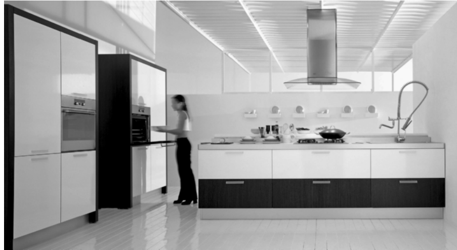
Figure 5-28 By placing the ovens side by side, access to the ovens can be designed to fit the cook's ergonomic profile. (Photo courtesy of NY LOFT.)
