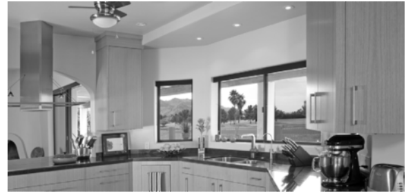
Figure 4-64 Ceiling light placement must always be carefully designed when ceiling fans are being used. (Photo courtesy of Mary Fisher Designs.com, Northlight Architectural Photography.com)
