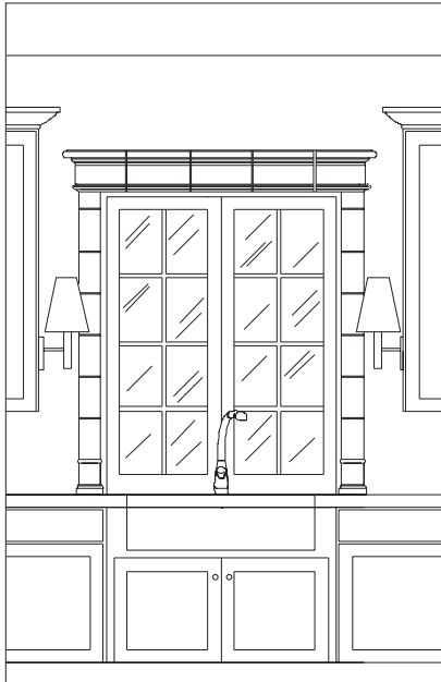
Figure i-1 A special stone-tile surround at a window affects the window size and placement, wall space on all sides, crown moldings and cabinetry adjacent to the window, window coverings, and lighting fixtures.
