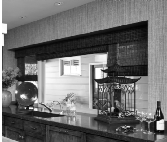
Figure 8-3 Sinks under windows can present a venting challenge. (Photo courtesy of Judy Svendsen, ASID, Raven Interiors/Mary Fisher Designs.com; Don Milici Photography)
