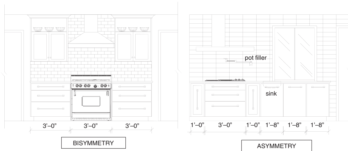
FIGURE 1-4 Bisymmetry is created with cabinets of equal size flanking the range and hood that are centered on the wall. Asymmetry is achieved by off-setting the cooktop and hood from center.
