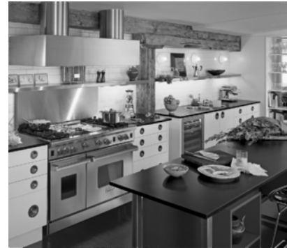
Figure 5-22 The high shelf can become a warm surface when the range is being used. It is a great place to warm plates before serving, but is not the place to store herbs and spices. (Photo courtesy of Sub-Zero/Wolf Photograph)
