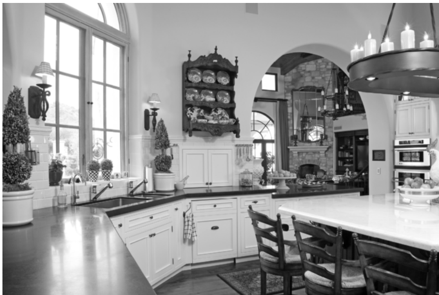
Figure 9-6 Chandeliers, ceiling lights, sconces, and track lighting systems are examples of surface-mounted fixtures. (Photo courtesy of Mary Fisher Designs.com, Northlight Architectural Photography.com)
