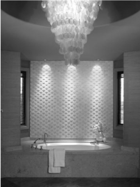
Figure 9-10 Wall-washing fixtures add visual interest as they illuminate a textured wall. (Photo courtesy of David Dalton, Inc., Los Angeles, CA 90019; www.daviddaltoninc.com )
