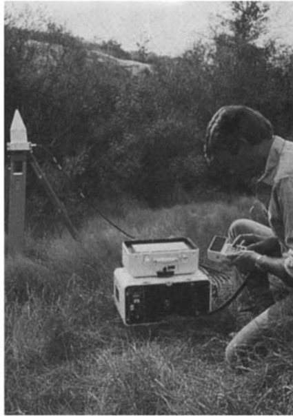
Figure 4.15 (b) Texas Instruments TI4100 dual-frequency GPS receiver with antenna and cassette tape recorder. (Texas Instruments).
