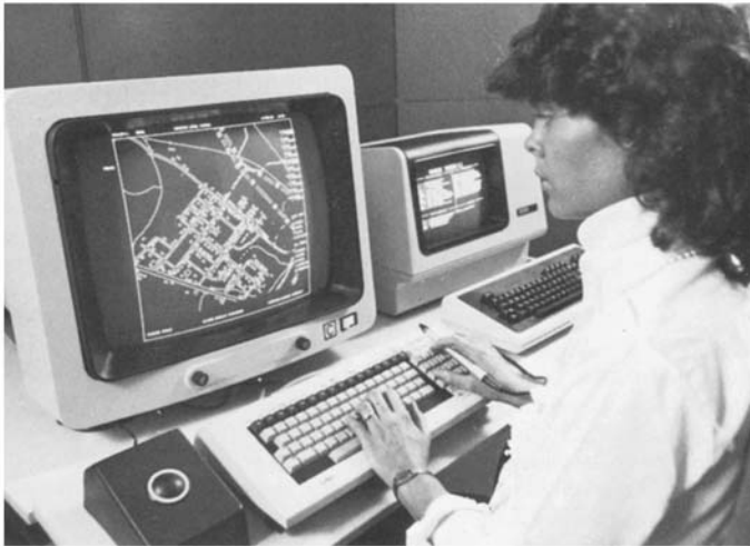
Figure 9.26 Graphics terminal utilizing vector refresh display.
