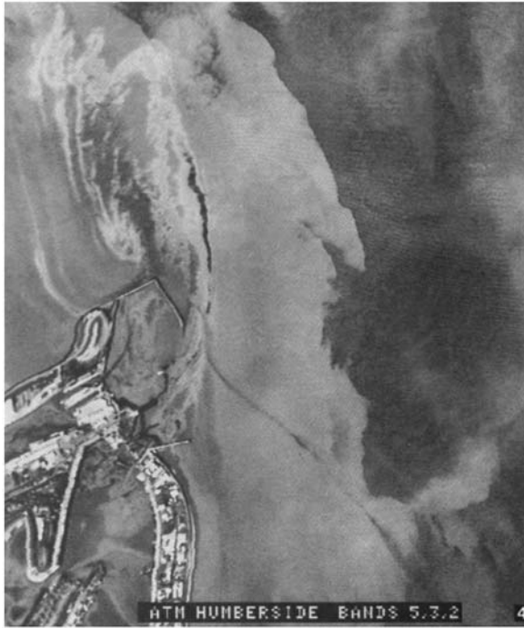
Figure 6.15 Airborne multispectral scanner image of the River Humber produced using the Daedalus AADS 1268 Airborne Thematic Mapper. Courtesy Hunting Technical Services Ltd.
