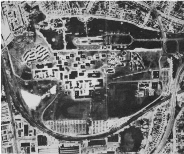
Figure 6.10 Thermal linescan image of the University of Surrey campus. Courtesy Clyde Surveys Ltd.
