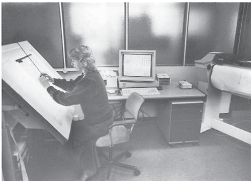
Figure 9.53 Interactive map editing station used in the OS digital field update system.
