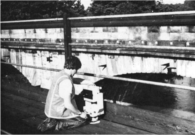
Figure 8.14 Railway viaduct being photographed with a Zeiss Jena UMK 10/1318 camera. Note targeted points on face of stonework.
