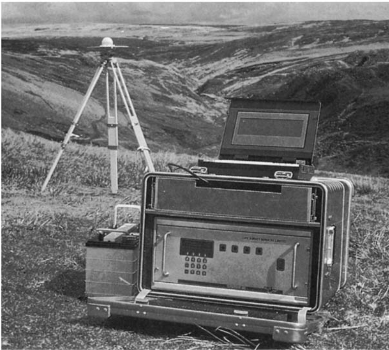
Figure 4.15 (a) Trimble 4000SX GPS receiver with antenna, power supply and data-logging computer. Courtesy GPS Survey Services Ltd.
