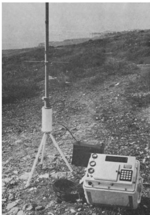
Figure 4.12 Magnavox 1502 TRANSIT Doppler receiver with antenna and power supply. From Stansell, T.A. (1978) The TRANSIT Navigation Satellite System , Magnavox, California, p. 25.
