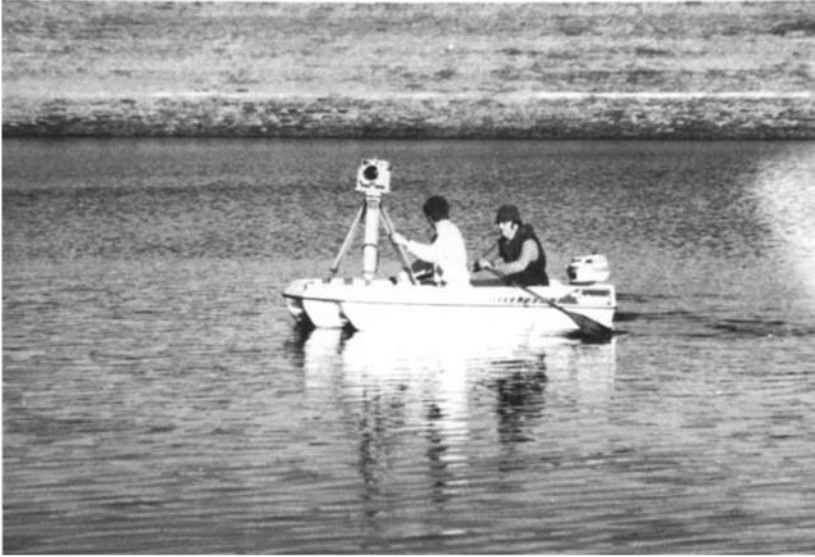
Figure 8.12 Zeiss Jena UMK 10/1318 camera mounted in a small dinghy, used to take photograph in Fig. 8.11.
