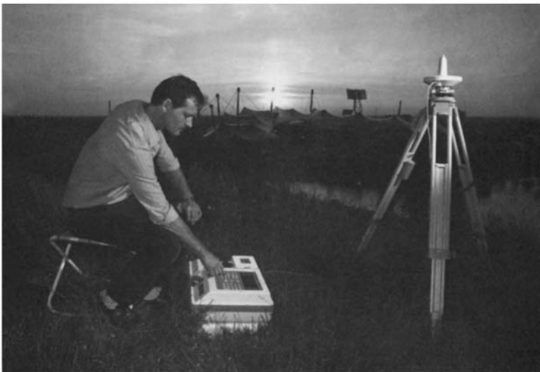
Figure 4.15 (c) Wild Magnavox WM101 GPS receiver with antenna and internal tape recording system. Courtesy Wild Heerbrugg (UK).
