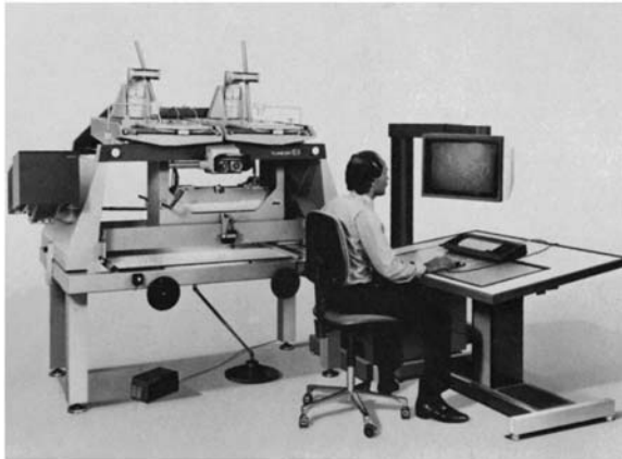
Figure 7.10 Zeiss Oberkochen Planimat with intergraph graphics display and interactive tablet digitizer (in foreground) and superimposition unit (mounted on the left side of the stereoplotting instrument).
