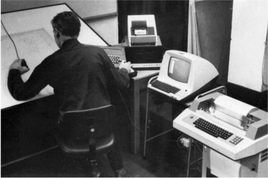
Figure 9.6 Blind digitizing using GTCO digitizer and tape cassette recorder.
