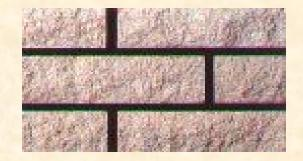
2. Face brick Brick made especially for exterior use with special consideration of color, texture and size, and used as a facing on a building. High durability.
