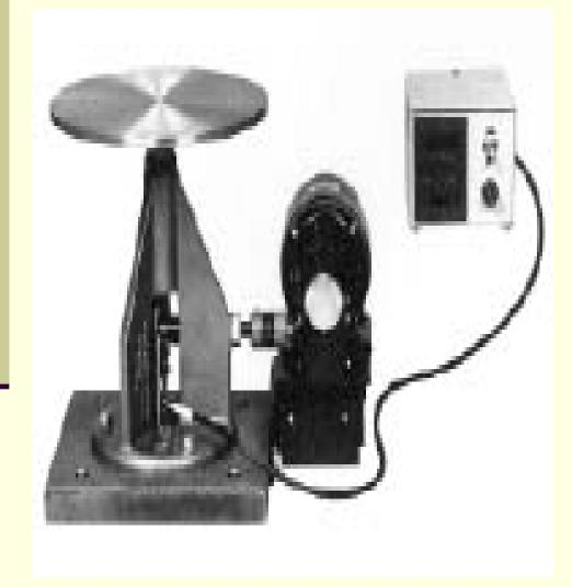
Determine the flow of cement pastes and cement mortars by measuring the spread in mm (width) of a standard cone on a dropping table. This value is a measure of the plasticity of the mortar.
