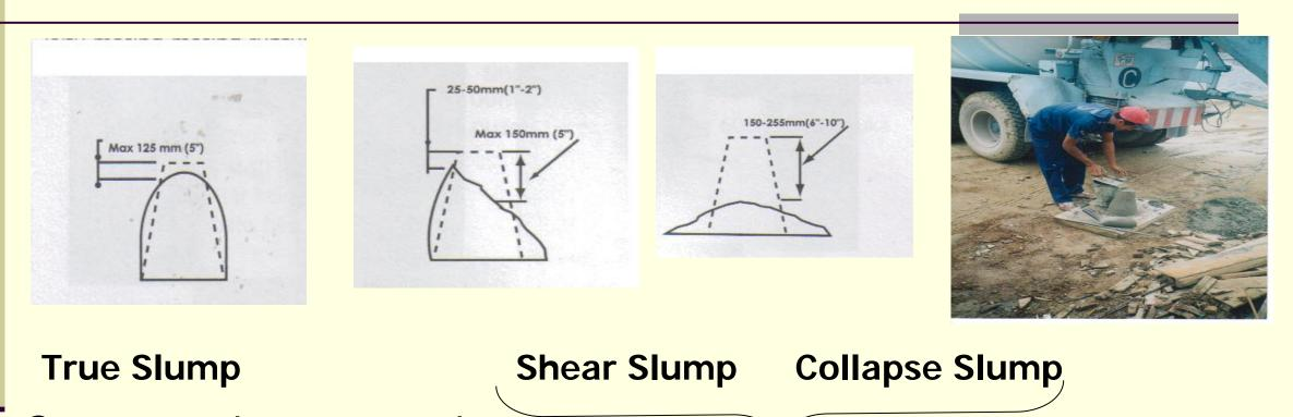
Concrete slump must be in this form. Normal slump Con range (12 mm – 115 mm) wet
