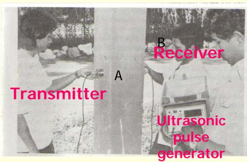
Time taken by the pulse to travel from point A to point B in concrete sample is recorded.
