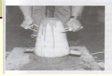
Cone is filled and level off. It is then carefully lifted.
