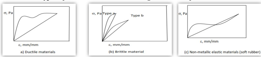
✓ Common types of nominal stress-strain diagrams are as follows:
