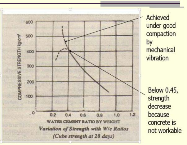
Variation of Strength with W/C ratio (Cube strength at 28 days)
