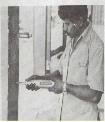
• The test is sensitive to the presence of aggregate and of voids immediately underneath the plunger.
