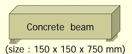
Measure the strength of an unreinforced concrete beam or slab to resist failure in bending
