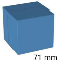
Mortar = Cement + Sand + Water 1 : 3 ( standard sand, one size and spherical shape) + Water (10% of the mass of dry materials)
