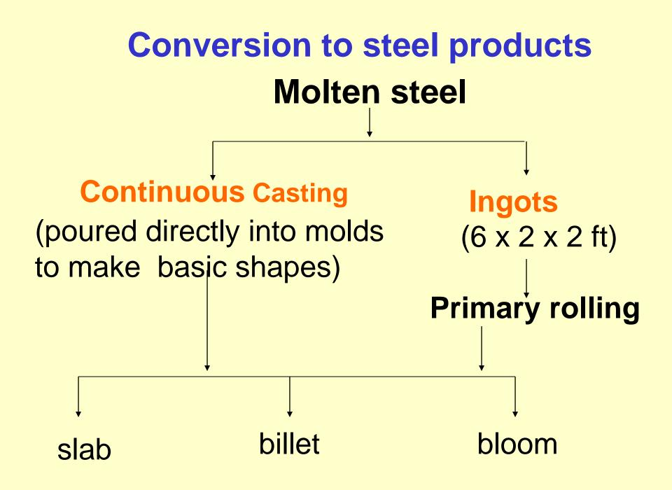
**SLAB.** Up to 3000 mm wide and up to 320 mm thick
