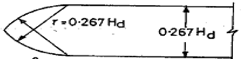
90° Cut water Nose pier, C_p=0.01
