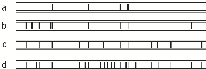
Figure 7. Positions of matrix cracks in a specimen (axial length 50 mm) of [0_2/90_8/0_2] T300-934 laminate loaded by tensile fatigue with the maximum cyclic stress 450 MPa at different moments of loading history: (a) 100 cycles, (b) 4 \times 10^3 cycles, (c) 10^5 cycles and (d) 2 \times 10^5 cycles. Vertical to horizontal scale 2:1,
