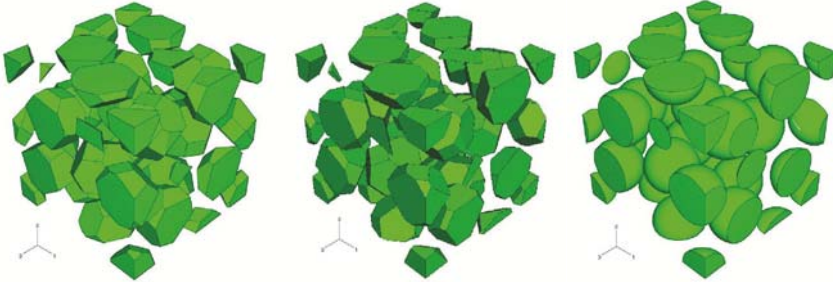
Figure 8. Three unit cells of nominal particle volume fraction \xi^{(i)} = 0.34 used for modeling the thermomechanical and thermal conduction behavior of diamond reinforced aluminum (Nogales and Böhm, 2008). The cells are referred to as UCDA (left), UCDB (center) and UCS (right).
