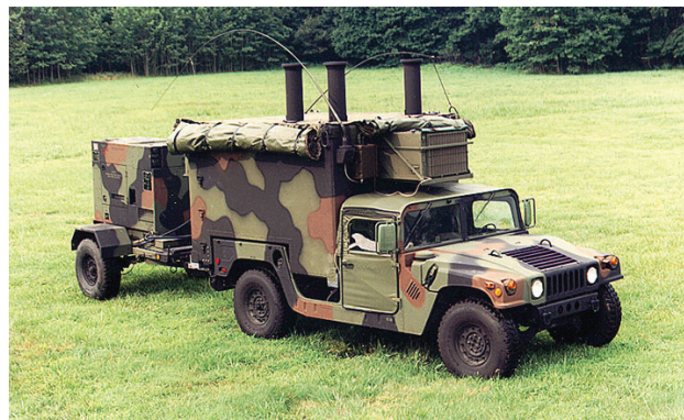
Fig. 20-1. The Biological Integrated Detection System (BIDS) is a semi-automated biological agent detection/identification suite mounted on a dedicated heavy high mobility multipurpose wheeled vehicle. The system uses multicomplimentary bio-detection technologies.
